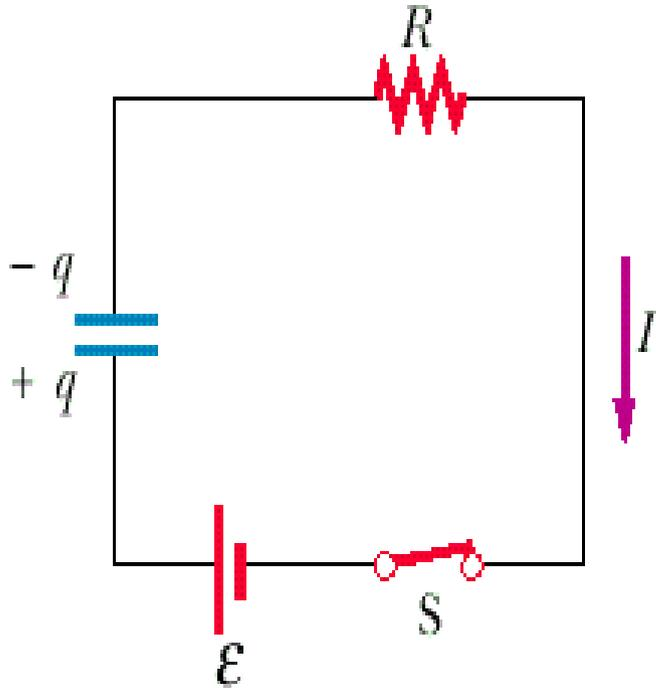
$$\frac{dq}{dt} = \frac{C\mathcal{E}}{RC} - \frac{q}{RC} = \frac{q - C\mathcal{E}}{RC}$$
