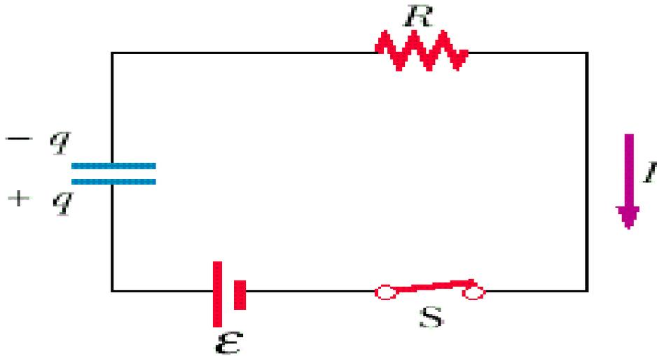
$$[\tau] = [RC] = \left[ \frac{\Delta V}{I} \times \frac{Q}{\Delta V} \right] = \left[ \frac{Q}{Q/\Delta t} \right] = [\Delta t] = T$$
