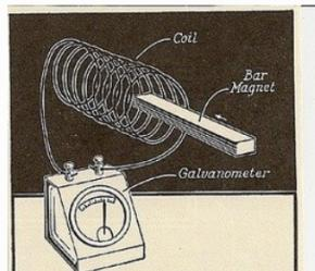
This is a simple representation of the principle of electromagnetic induction, discovered by Faraday. Can you explain the meaning of this diagram?
