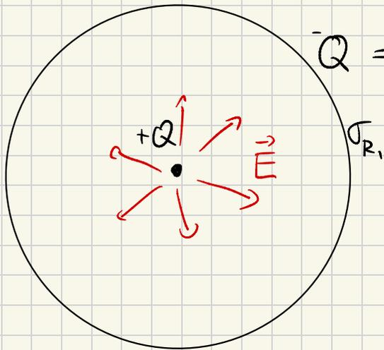
$$-Q \Rightarrow \sigma_{R_1} = \frac{-Q}{2\pi R_2 L}$$
