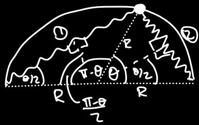
$$V(\theta) = V_{\text{resorte},1} + V_{\text{resorte},2}$$
