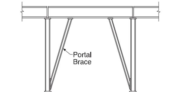
Fig. 17.2.4 Portal Crane Runway Bracing
