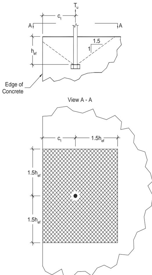
Fig. 9.1.3 Breakout Cone in Tension Near an Edge
