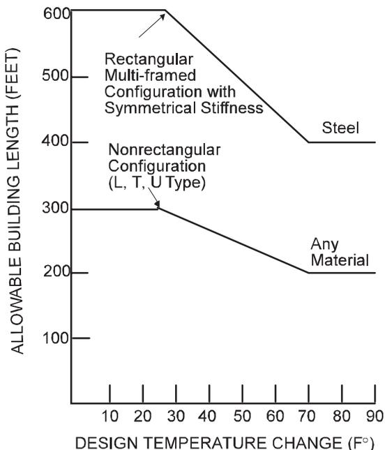
Fig. 4.4.1 Expansion Joint Spacing Graph
