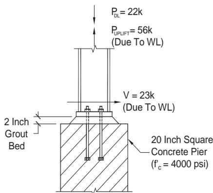
Fig. 9.4.4 Column pier support
