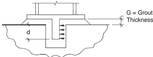
Fig. 9.4.7 Shear Lug Depth
