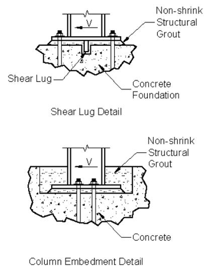
Fig. 9.3.1 Transfer of Base Shears Through Bearing
