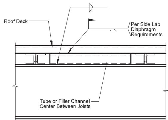
Fig. 8.2.3 Shear Collector
