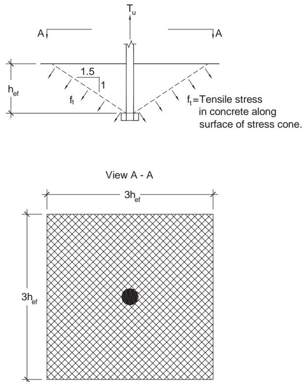
Fig. 9.1.1 Full Breakout Cone in Tension per ACI 318-02
