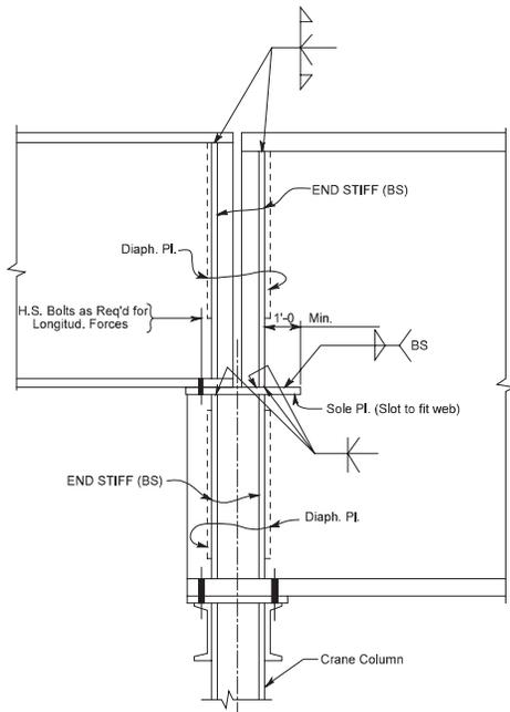
Fig. 18.2.6 Section at Different Depth Crane Girders
