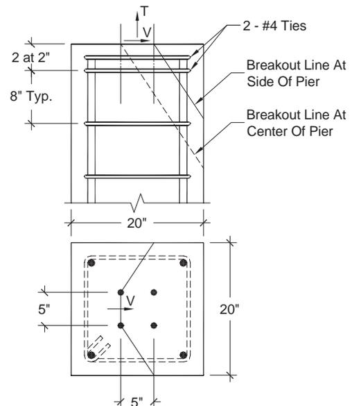
Fig. 9.4.5 Pier for Ex. 9.4.2 Showing Shear Breakout Cone
