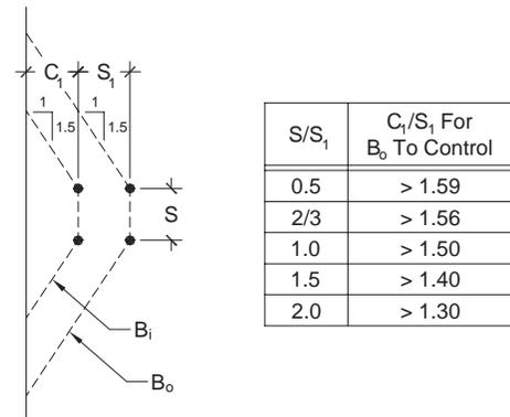
Fig. 9.2.2 Concrete Breakout Surfaces for Group Anchors
