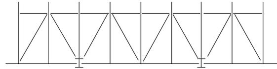
Fig. 20.1.4 Horizontal Bracing
