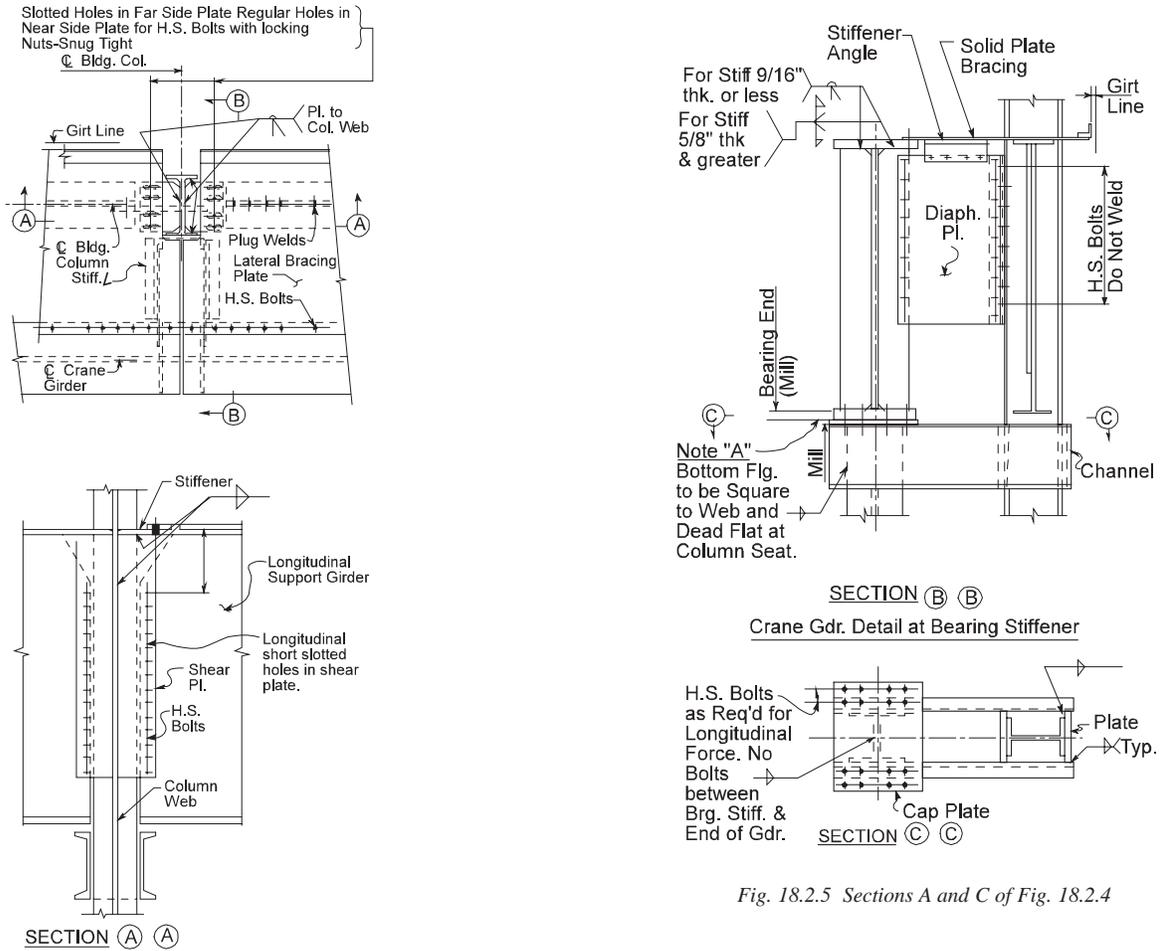
Fig. 18.2.5 Sections A and C of Fig. 18.2.4
