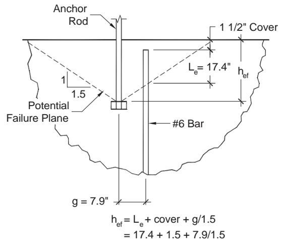
Fig. 9.4.3 Embedment Depth for Transfer to Reinforcing Bars
