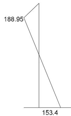
Fig. 20.2.5 Column Moments Using Fig. 20.2.4 Equations
