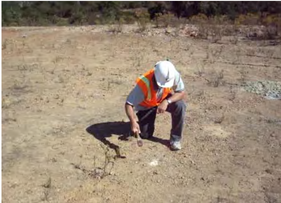
Figure 15.11. Using a small sledge hammer as a wave source for the SASW test. In addition, a larger, 10-lb sledge was also used as a wave source.
