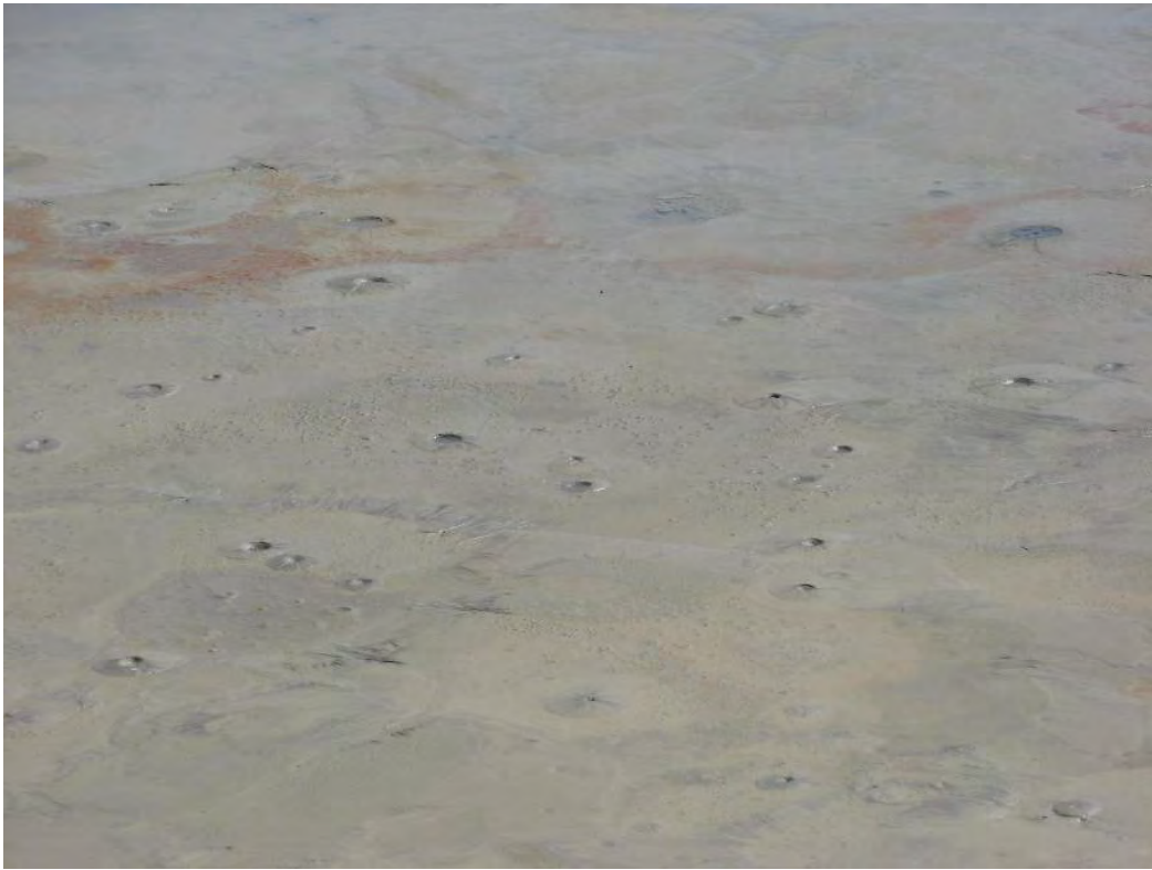
Figure 11.11. March 9, 2010 Sand Boils in Tailings about 10 m Upstream of Ovejeria Tailings Dam (S33.052016°, W70.798687°)
