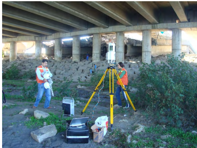
Figure 15.14 Terrestrial laser scanning with a Riegl z420 LIDAR unit at the West Bio Bio River (Juan Pablo 2) bridge.
