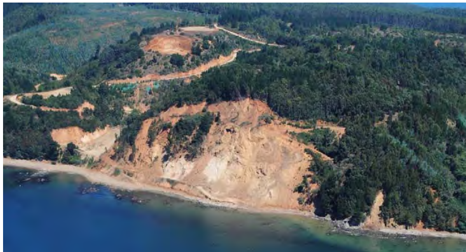
Figure 10.13. Disaggregated landslide complex, Punta Tumbes looking West (36.66°S, 73.098°W).
