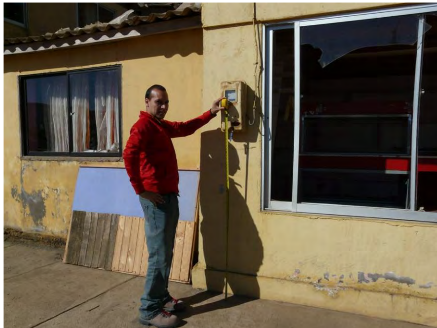
Figure 13.28. Tsunami flow depths reached a minimum of 1.5 m along the waterfront in Bucalemu (S34.641882° W72.043158°, 1051 hrs on 03/15/2010).
