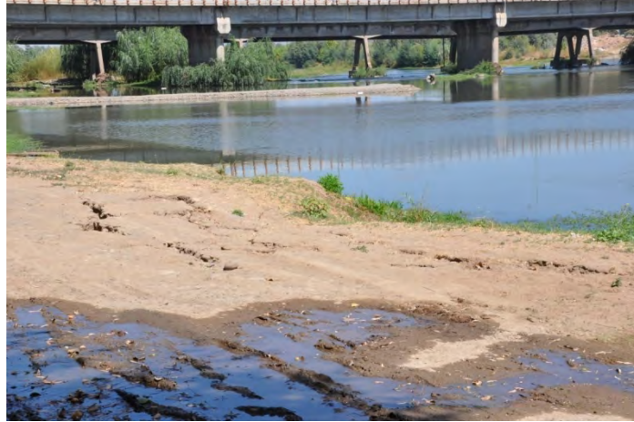
Figure 9.33. Near shore lateral spread on the western shore of the Rio Claro in Talca, view looking south. (S35.419682°, W71.682359° on 3/18/2010). Both the pedestrian and vehicular crossing bridges are shown in the background.
