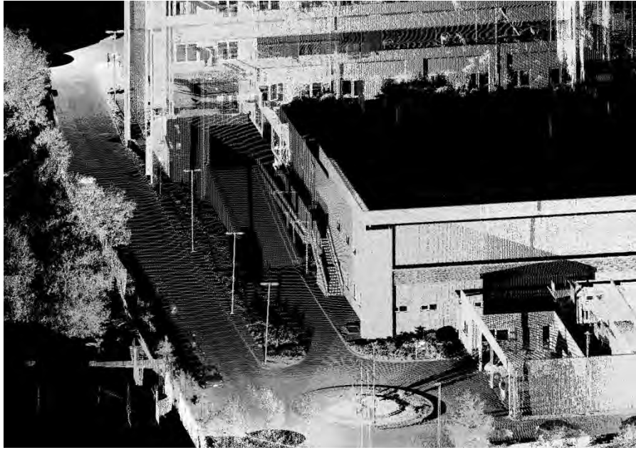
Figure 15.44. Oblique view of the north east side of Provincial Hospital of Curanilahue, 37.47352°S, 73.34824°W. The SASW test was performed along the three light posts above the circle.
