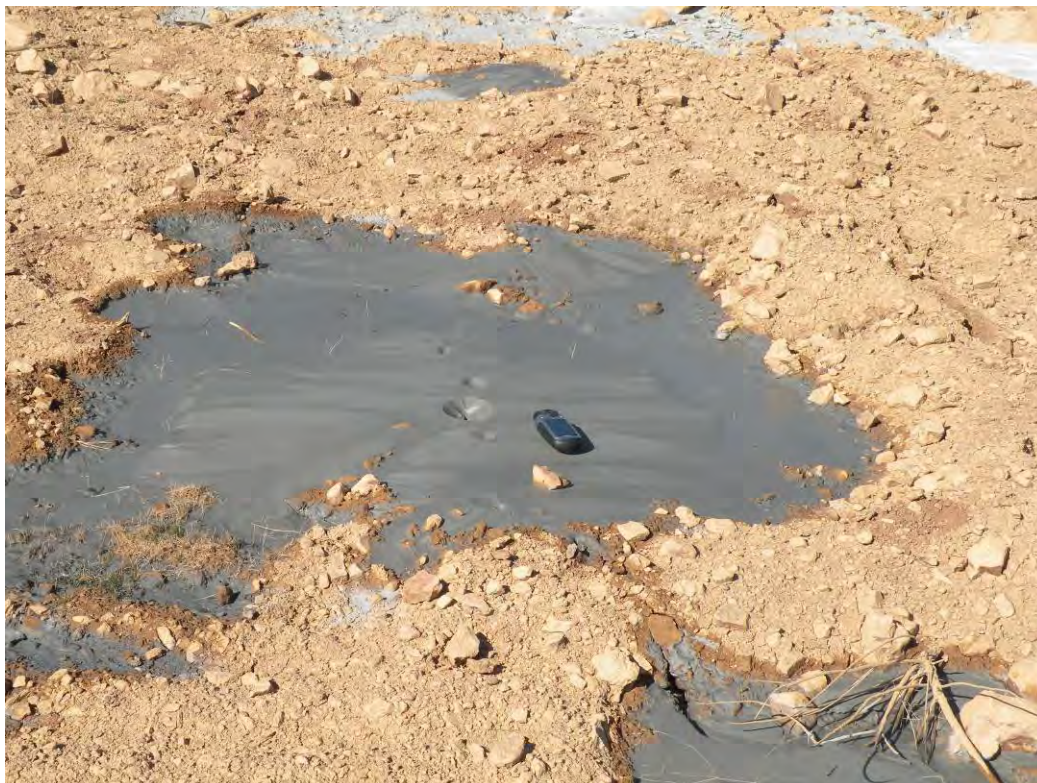
Figure 11.33. March 11, 2010. Tailings Sand Boil Due to March 11, 2010 M6.9 Earthquake near Rancagua ( S35.184146^{\circ} , W71.761118^{\circ} )
