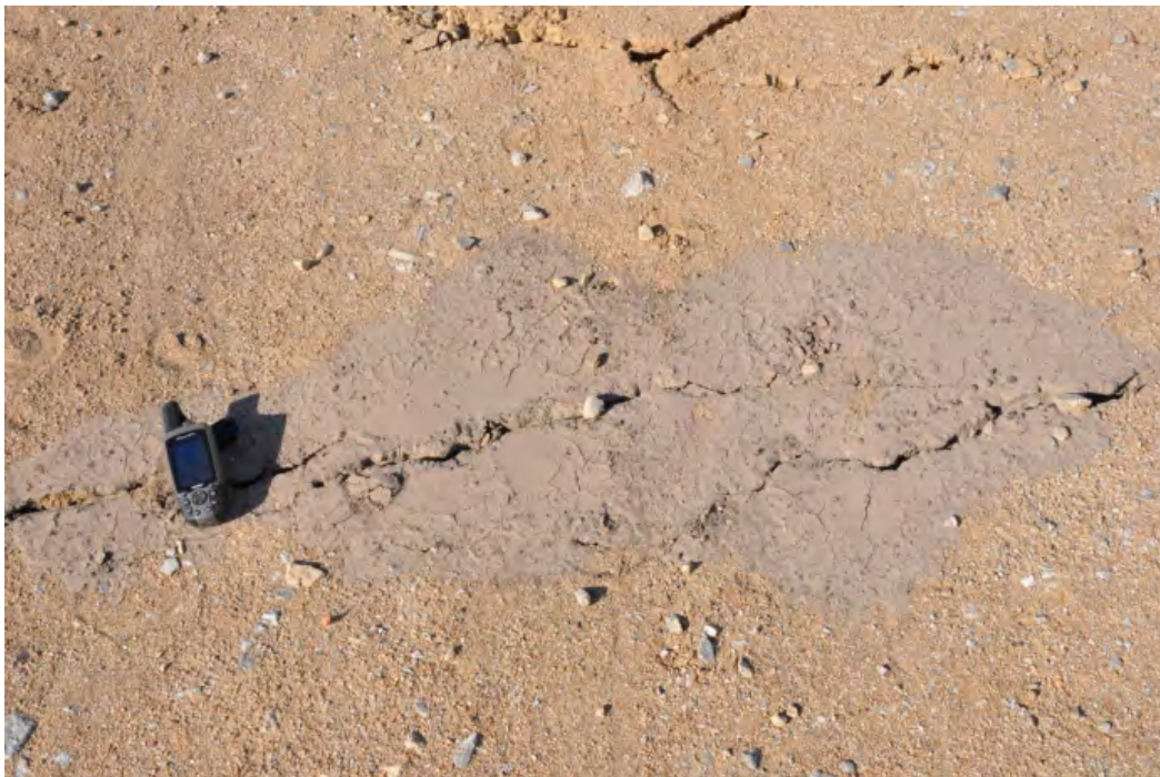
Figure 6.7. Liquefaction boils in undeveloped land area along west shore of Tres Pascuales lagoon in Concepcion (S36.8155°, W73.0460°; 3/14/2010)
