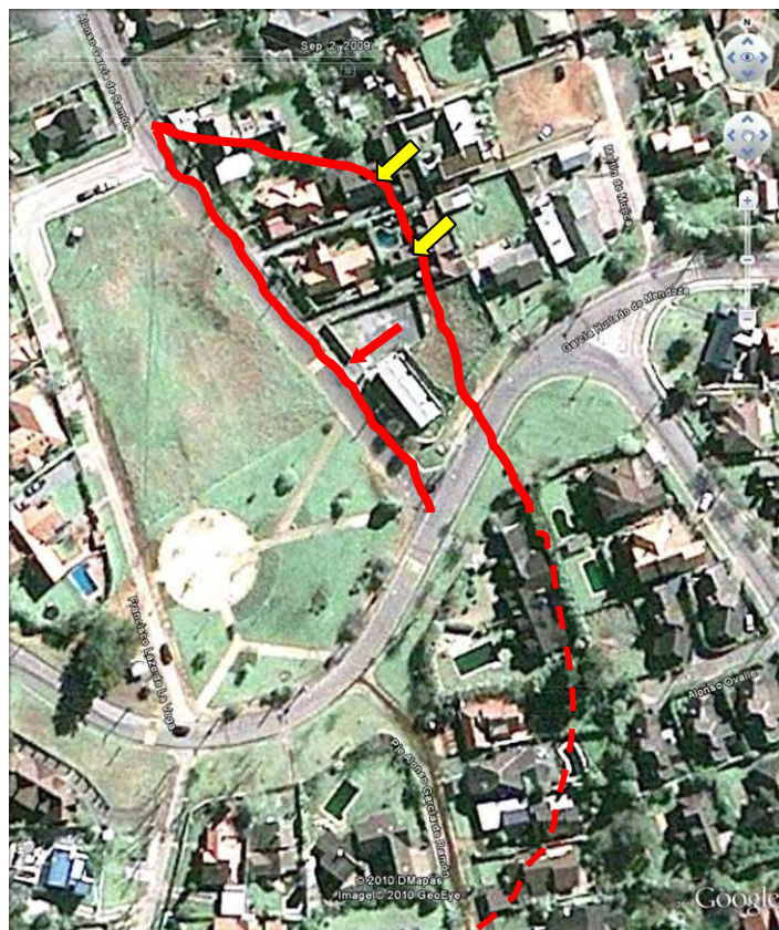
Figure 7.29. Affected area with approximate limits of the translational earth movement; the toe of the slide is along the eastern side of Alonso García de Ramón Road and the head scarp runs through the houses and the open field behind the rectangular apartment complex. (S36.791841°, W73.056996°). The yellow arrows denote the location of two severely damaged home which are shown in Figure 7.31.
