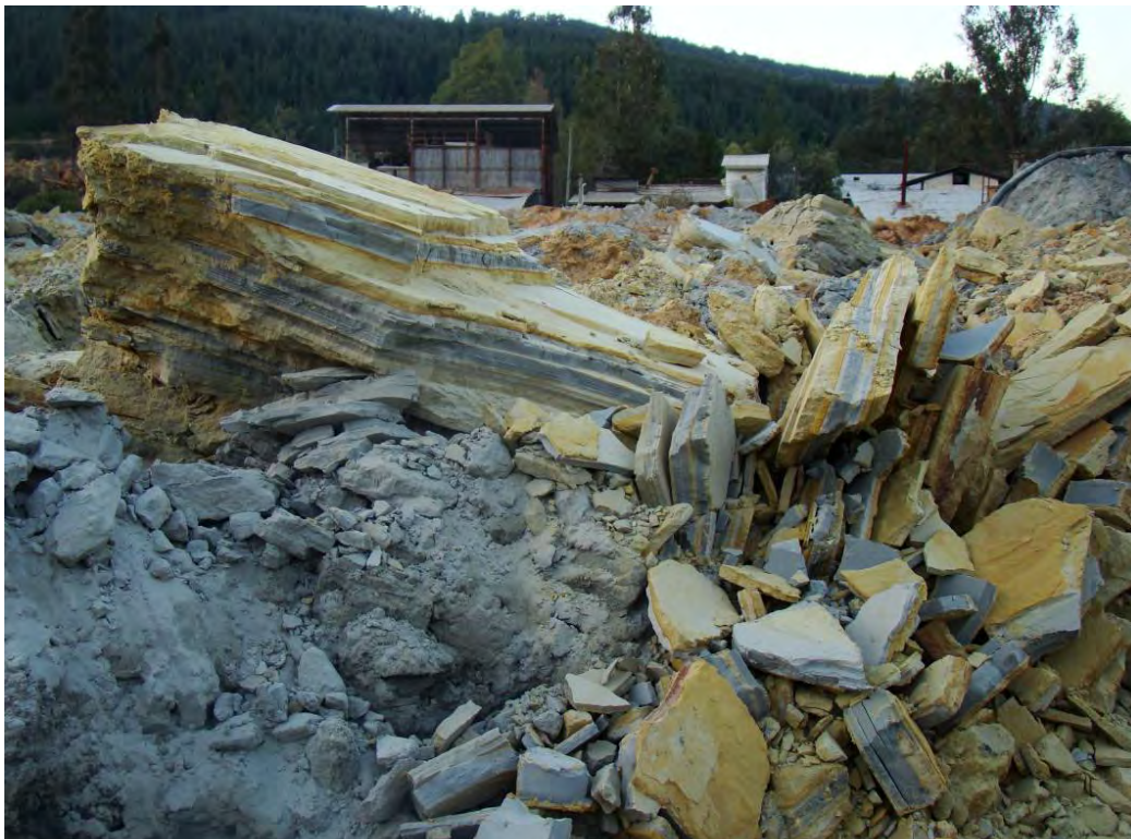
Figure 11.30. March 11, 2010. Variably Oxidized Tailings – Unsaturated Conditions in Upper Portion of Tailings Impoundment (S35.18728°, W71.75781°)
