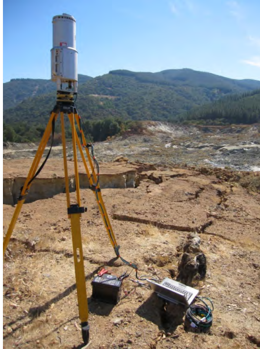
Figure 15.13 Terrestrial laser scanning with a Riegl z420 LIDAR unit at the Las Palmas Mine tailings dam failure. The system uses a PC for data acquisition and a car battery to power the laser.
