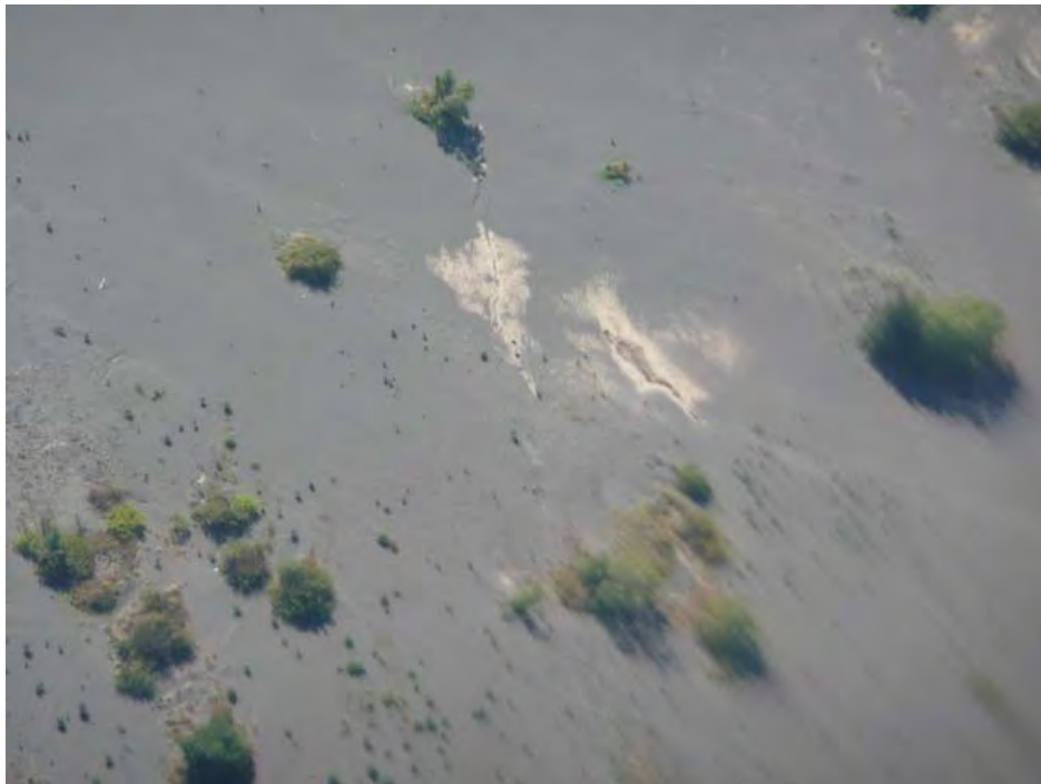
Figure 6.5. Lower elevation view of fissures and liquefaction ejecta. This was taken along the lower Rio Bio Bio near Concepcion ( \sim S36.8239°, \sim W73.0944°, 15:00, 3/6/2010). The dark surface sediment is from the Rio Laja that intersects the Bio Bio approximately 20-30 km upstream from this point. The light ejected sediment is supplied by the main stem of the Rio Bio Bio upstream of the Rio Laja.
