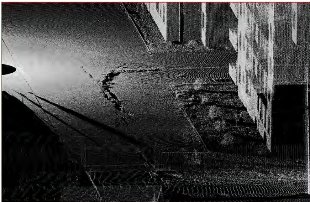
Figure 15.35. Detailed LIDAR imagery of settlement of soil around the Riesco Building (Southwest).
