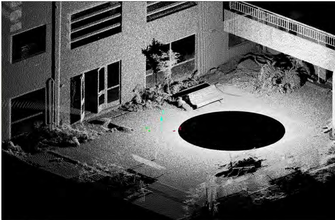
Figure 15.45. Oblique view of the east courtyard of the Provincial Hospital of Curanilahue, 37.47352°S, 73.34824°W. Liquefaction induced structural settlement is clearly evident along the courtyard perimeter.
