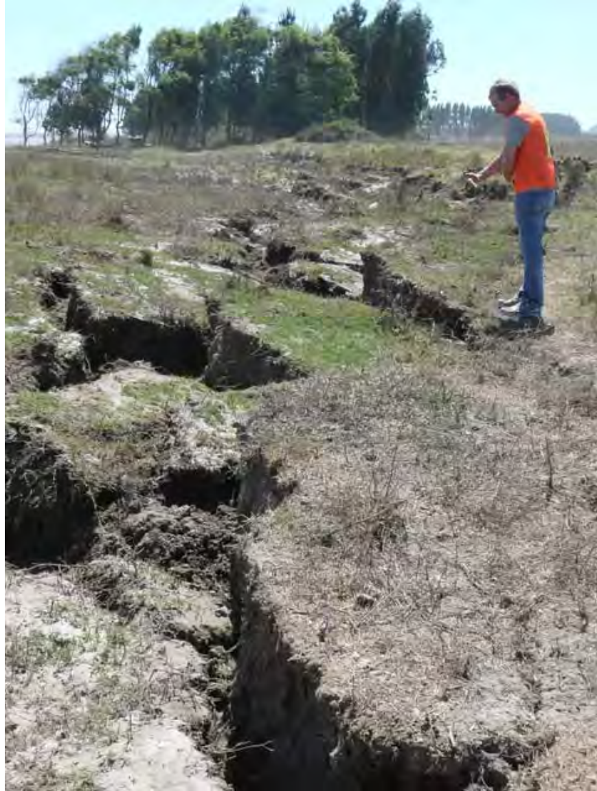
Figure 6.6. Lateral spreading blocks translated and rotated towards the river. This picture shows Keith Kelson standing on the north bank of the Mataquito River downstream of the coastal highway bridge (S3505078°, W72.16240°, 11:00, 3/8/2010).
