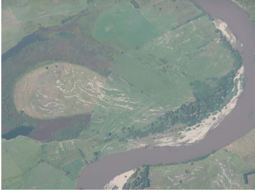
Figure 6.4. Liquefaction ejected and lateral spreading features observed along Carampangue River towards the southern extents of damage ( \sim S37.2780°, \sim W73.2541°, 17:00, 3/6/2010).
