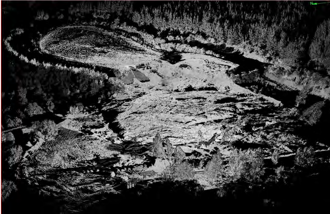
Figure 15.54 Oblique LIDAR view of the Las Palmas Tailings Pond Failure, Talca (35.184679° S, 71.759410° W). The tailings pond head scarp is in the upper-left. The toe of the slide is in the line of trees at the bottom right.
