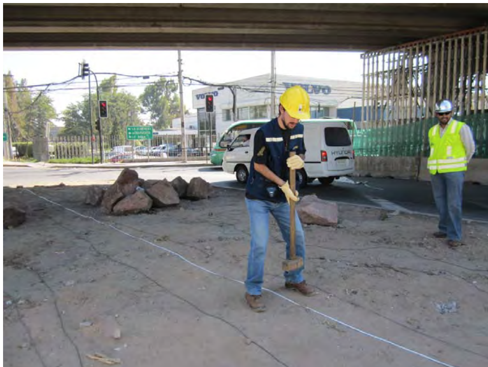
Figure 15.60 SASW line and test, Bridge Ring 3 “Lo Echevers” Bridge, Santiago, 33.376159°S, 70.747742°W, April 13, 2010
