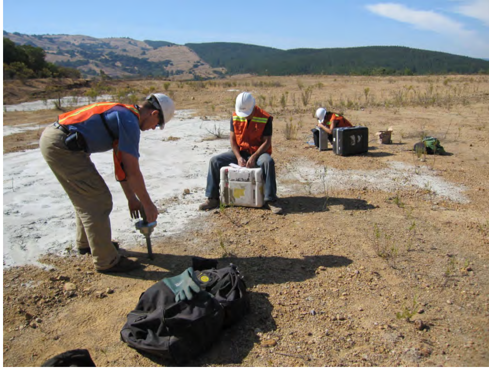
Figure 15.10. When the DCPT test was penetrating the upper two meters of soil, the drop weight was used as a wave source for the SASW test. (35.183884°S, 71.76110°W; 28 March 2010;
