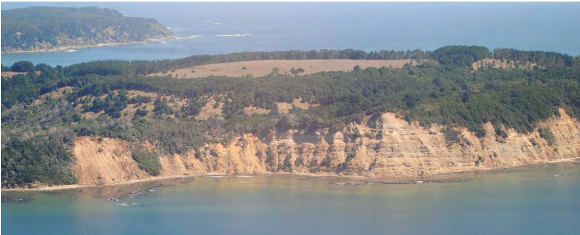
Figure 10.12. Shallow failures and raveling in Tertiary sedimentary rocks on Isla Quiriquina (36.627°S, 73.05°W).
