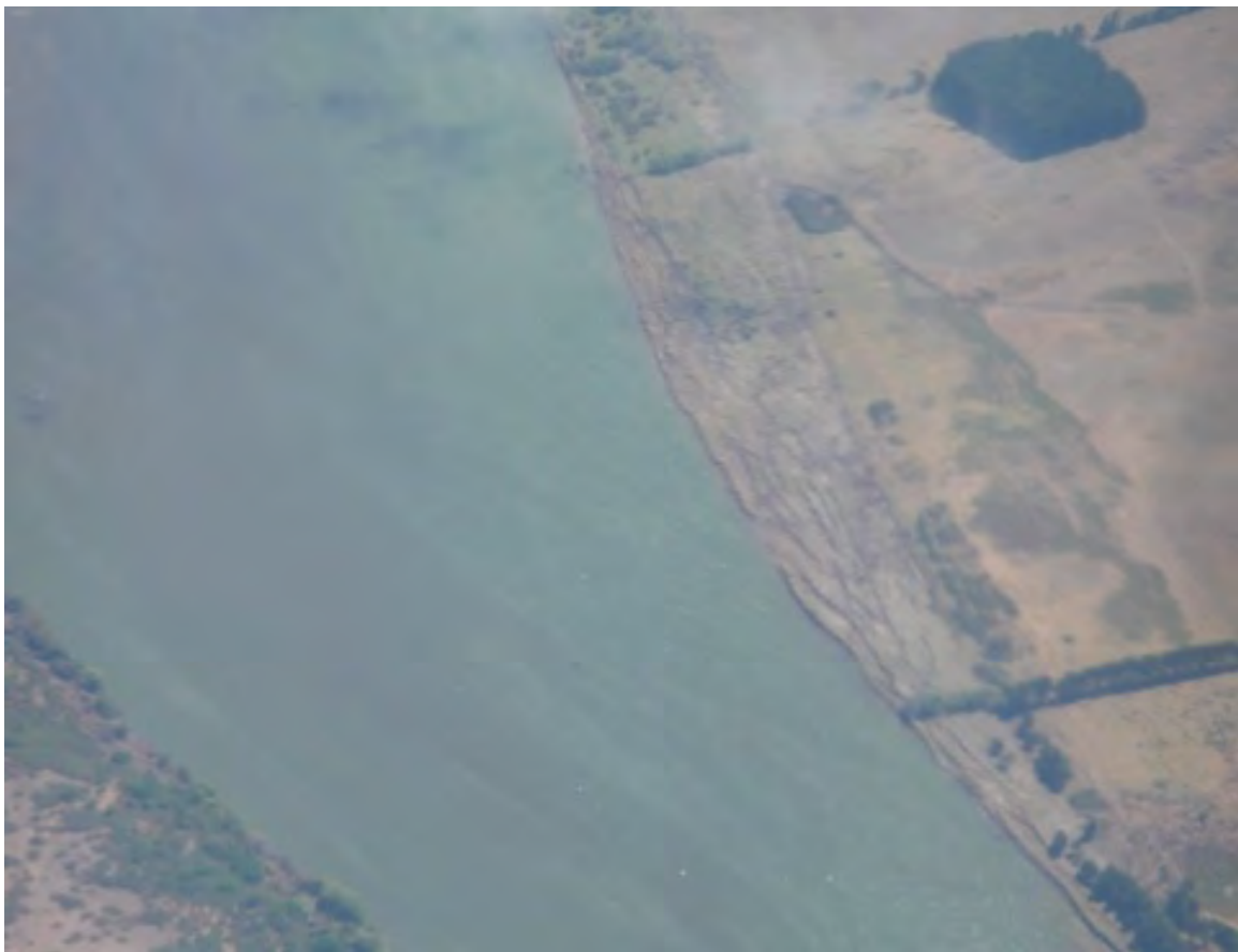
Figure 6.3. Lateral spreading feature observed along Rio Maipo towards the northern extents of damage (S33.9913° W71.5316°, 12:30, 3/6/2010).
