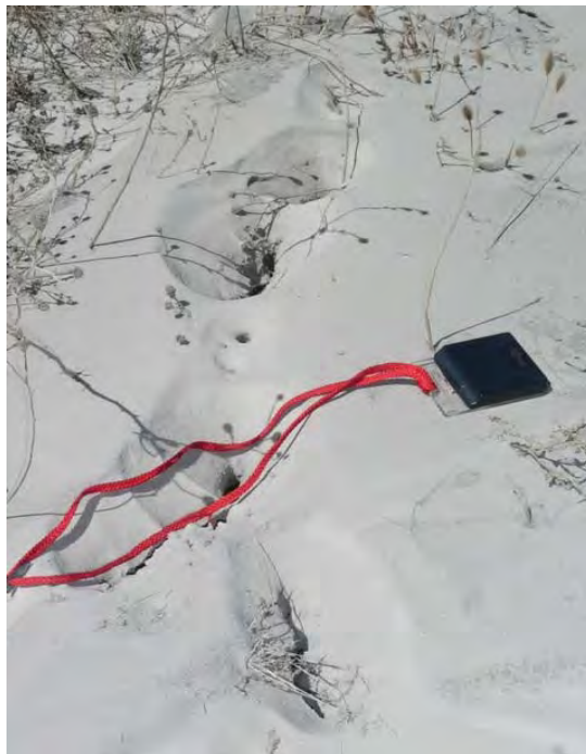
Figure 6.14. Typical liquefaction ejecta found at Mataquito bridge (S3505078°, W72.16240°, 11:00, 3/8/2010). The ejecta consisted of medium to fine sand with some fines.
