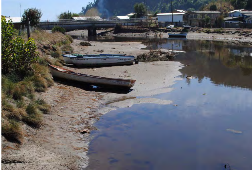
Figure 4.13. Ground view looking north in village of Laraquete, from the highway bridge toward the estuary outlet. Fishing boats stranded on left bank; tsunami high water mark approximately at the bank crest. Light, wooden-frame residences on both banks were unaffected by tsunami waves confined within existing tidal channel. Local witness indicated that the sea level went down about 0.5 m after the earthquake, and that the estuary bottom had not been exposed before (i.e., uplift of about 0.5 m). (S37.166661° W73.184481°; 1238 hrs on 03/10/2010)
