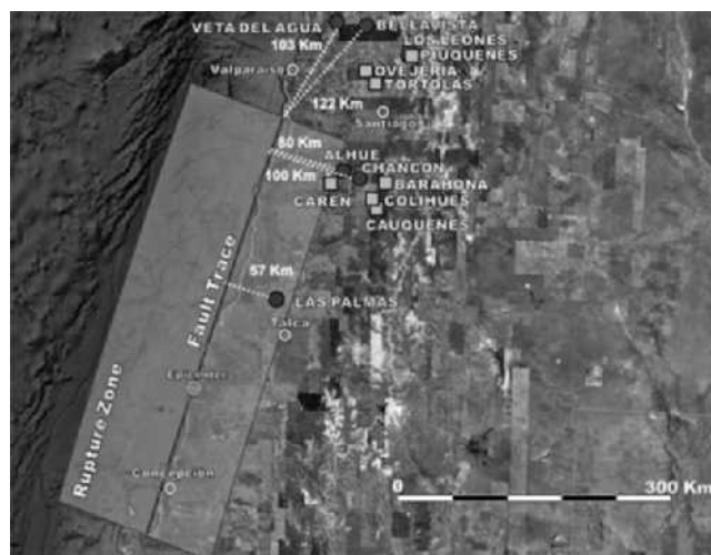
Figure 17. Large tailings dams with stable response (square) and tailings dams that experienced seismic failures during 2010 Maule Earthquake (circles).
