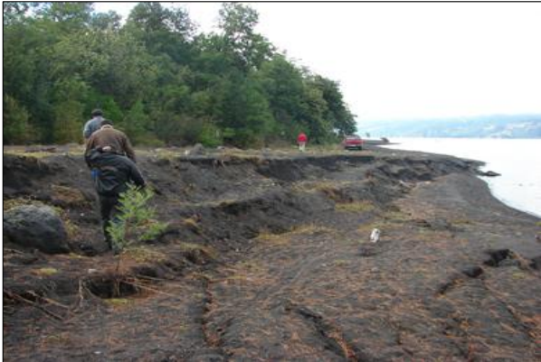
Fig. 10.- Lateral Spreading observed in an area of low intensity: Pocura and Calafquen (source: Sernageomin and Municipalidad of Panguipulli)
