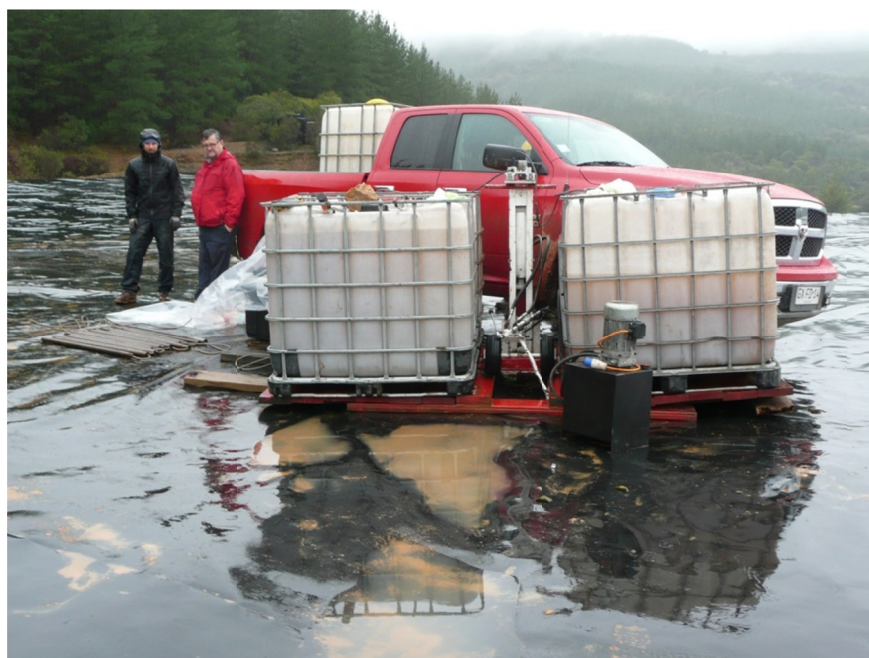
Figure 5.1 Portable “ramset” mobilized for Las Palmas field investigations because of the difficult access conditions. The reaction weight was provided by water tanks and truck. The ramset is the white hydraulic jack in the middle. The black box with orange cord to the right is the hydraulic pump.
