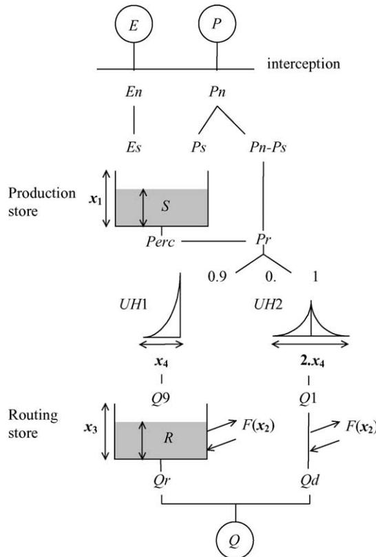
Fig. 1. Diagram of the GR4J rainfall-runoff model.
