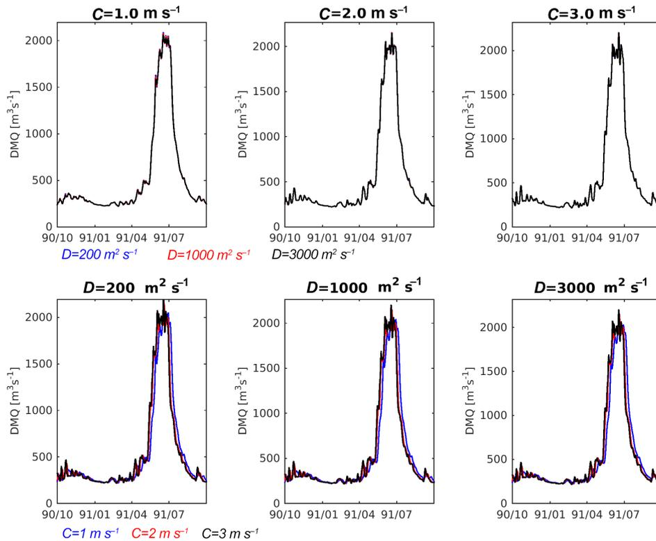
**Figure 9.** Sensitivity of simulated runoff at Colorado River at Lees Ferry (location B in Fig. 5) to IRF-UH parameters. The top panels show sensitivity to diffusivity  $D$  with three fixed celerity  $C$  values (from left to right:  $C = 1.0, 2.0,$  and  $3.0 \text{ ms}^{-1}$ ). The bottom panels show sensitivity to celerity  $C$  with three fixed diffusivity  $D$  values (from left to right:  $D = 200, 1000,$  and  $3000 \text{ ms}^{-2}$ ).
