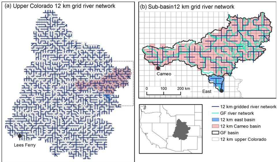
**Figure 10.**  $1/8^\circ$  ( $\sim 12$  km) grid-based river network for the upper Colorado River basin (a) and two sub-basins inside the upper Colorado–Colorado River near Cameo and East River at Almont (b). HRUs for each GF river segment are not shown for clarity in (b).
