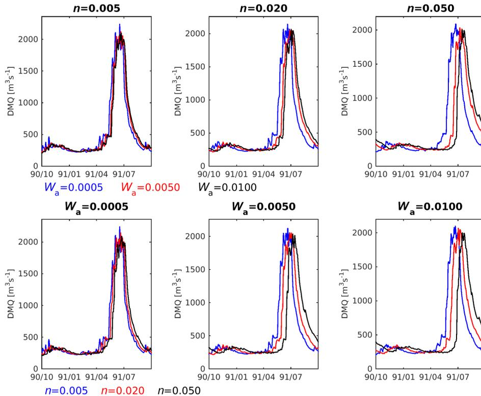
**Figure 8.** Sensitivity of simulated runoff at Colorado River at Lees Ferry (Location B in Fig. 5) to the two KWT parameters. The top panel shows sensitivity to width factor  $W_a$  with three fixed Manning coefficients  $n$  (from left to right:  $n = 0.005, 0.02, \text{ and } 0.05$ ). The bottom panel shows sensitivity to Manning coefficient  $n$  with three fixed width factor  $w$  (from left to right:  $W_a = 0.0005, 0.0050, \text{ and } 0.0100$ ).
