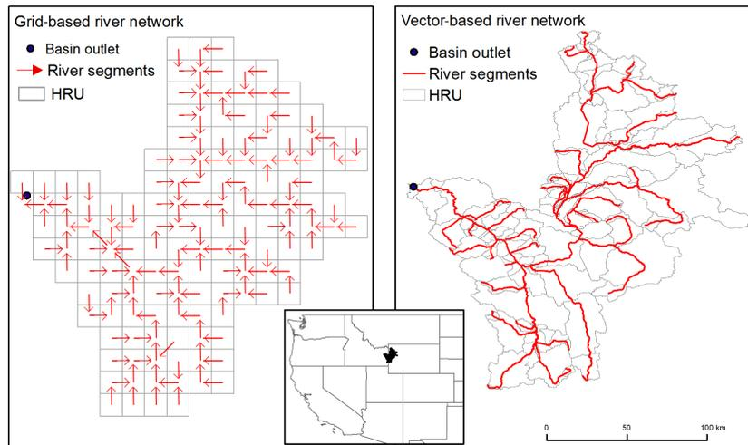
**Figure 1.** Comparison of  $1/8^\circ$  ( $\sim 12$  km) gridded river network and vector river network from United States Geological Survey (USGS) Geospatial Fabric for the upper part of Snake River basin (Viger, 2014).
