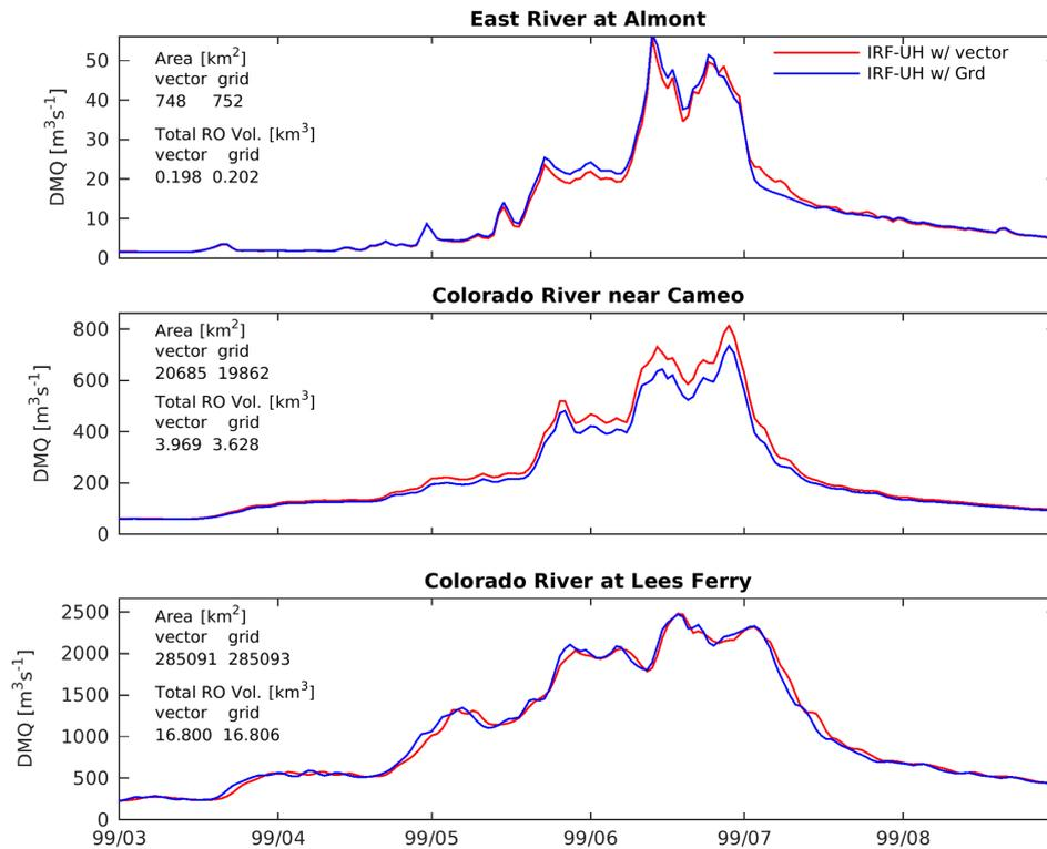
**Figure 11.** Comparison of IRF-UH routed flow with two river networks ( $1/8^\circ$  grid-based river network and GF vector-based river network) at three locations in the upper Colorado River basin (See Fig. 10 for river network and basin boundaries).
