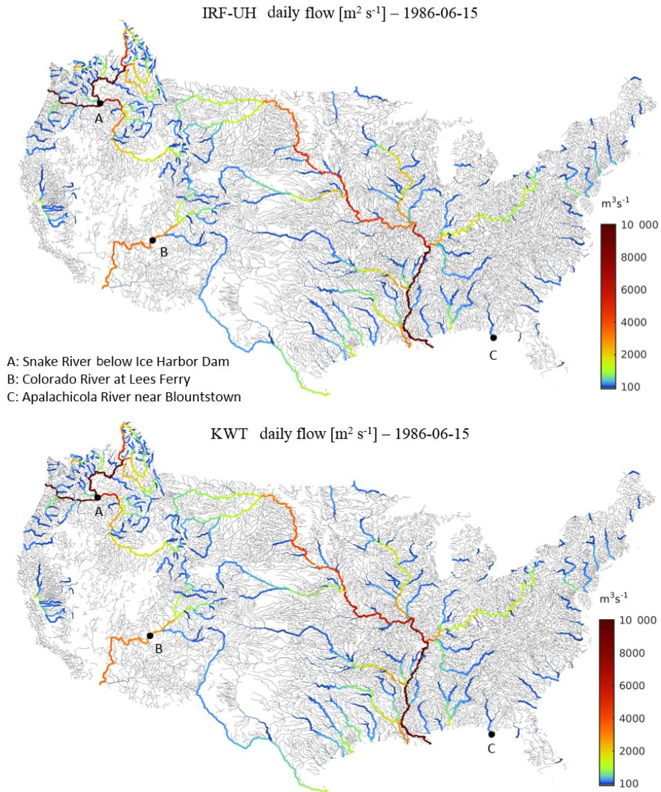
**Figure 5.** Spatially distributed daily streamflow on 15 July 1986 in the GF river network simulated with mizuRoute. Gray lines indicate flow less than  $100 \text{ m}^3 \text{ s}^{-1}$ . The streamflow time series shown in Fig. 6 are extracted at three USGS gauges A–C.
