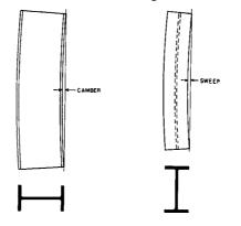
Positions for Measuring Camber and Sweep of W and HP Shapes
