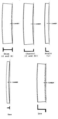
Positions for Measuring Camber of Shapes
