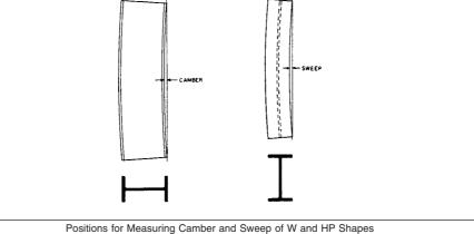
Permitted Variation in Straightness, in.  $\frac{1}{8}$  × (number of feet of total length/10)<sup>A</sup> Camber and sweep When certain sections<sup>B</sup> with a flange width approximately equal to depth are specified in the order for use as columns: Lengths of 45 ft and under  $\frac{1}{8} \times (\text{number of feet of total length/10})$  but not over  $\frac{3}{8}$ Lengths over 45 ft  $\frac{3}{8} + \frac{1}{8} \times ([number of feet of total length - 45]/10)]$
