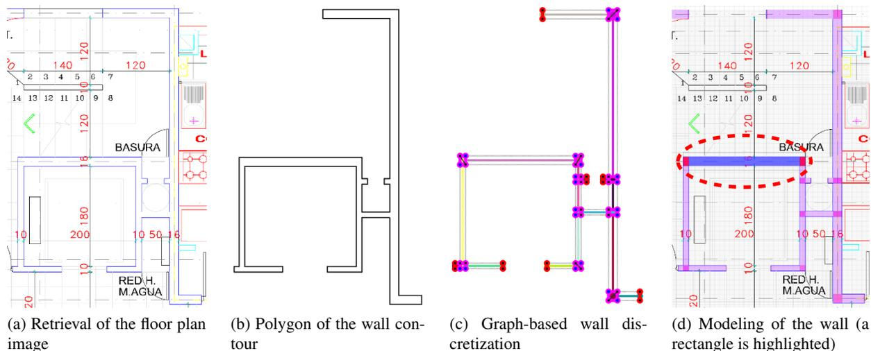
**Figure 3:** Example of the walls’ assembly process.
