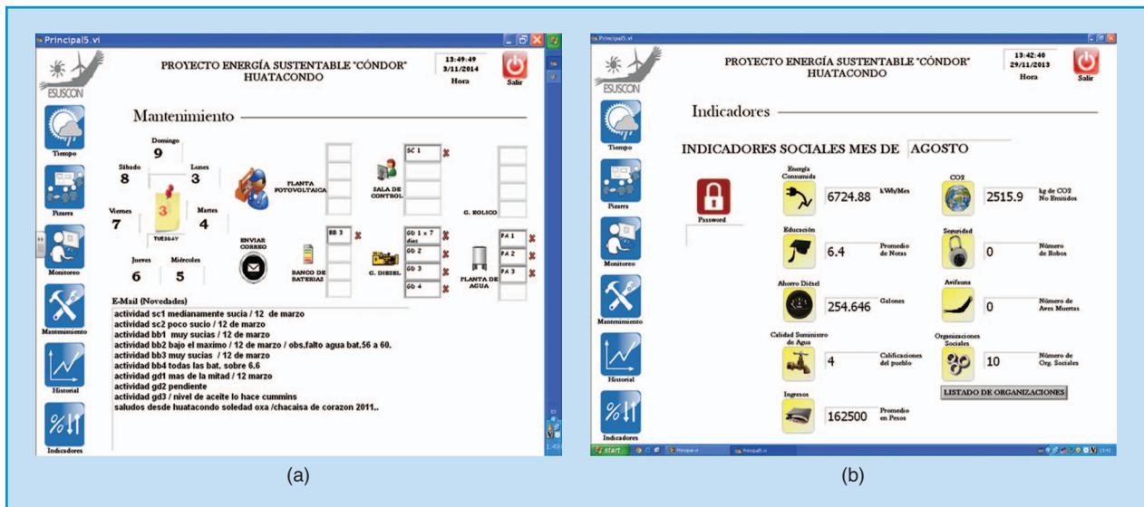
**figure 9.** The HMIs for (a) maintenance management and (b) sustainability indicators. The HMIs are presented in Spanish, as they were designed for the Huatacoondo community's use.
