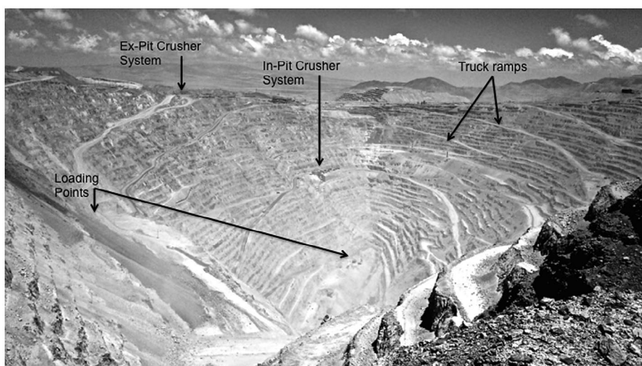
Figure 1. Current Chuquicamata operating configuration showing relative locations of equipment.
