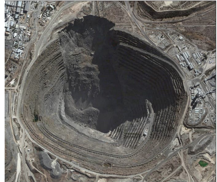
Caving induced failure in Palabora Mine, South Africa
