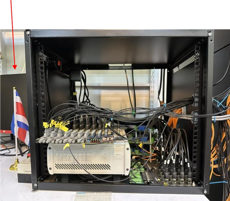
Dspace controller, optical board and 21 (LEM) voltage transducers
