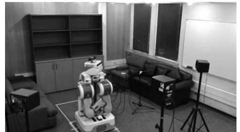
Figure 2: The experimental setup used to record RIRs.
