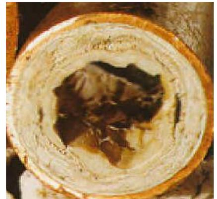
fig 2. Gypsum precipitates around in a well.
