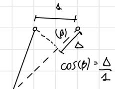
$$K_{22} = \frac{12EI}{3^3} \times 2 + F_{b2} \cos(\beta) = \frac{24EI}{27} + \frac{EA}{6,7} \left( \frac{6}{6,7} \right)^2 \quad \left. \begin{array}{l} K_{22} = 1441 \left[ \frac{\text{tonf}}{\text{m}} \right] \\ K_{21} = -1441 \left[ \frac{\text{tonf}}{\text{m}} \right] \end{array} \right\}$$
