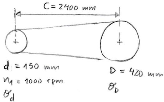
$$V = \frac{\pi d n_1}{60} = \frac{\pi \left(\frac{150}{1000}\right) 1000}{60} = 7.854 \frac{\text{m}}{\text{s}} \quad \left. \right\} \quad (1)$$
