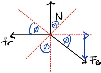
$$\begin{aligned} \hat{x} \downarrow & F_e \cos \phi - f_r = M \cdot a_x \\ \hat{y} \downarrow & N - F_e \sin \phi = M \cdot a_y \end{aligned}$$
