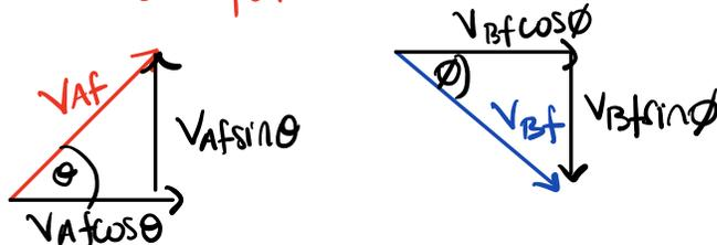
$$\Rightarrow \vec{p}_f = mV_{Af} \cos \theta \hat{x} + mV_{Af} \sin \theta \hat{y} + mV_{Bf} \cos \phi - mV_{Bf} \sin \phi$$
