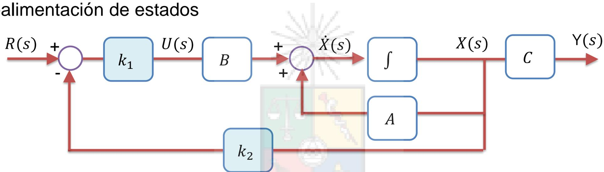
$$\begin{aligned} \dot{x} &= Ax + Bu \\ y &= Cx \\ u &= k_1(r - k_2x) \end{aligned}$$
