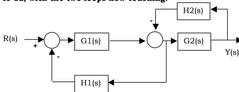
Working algebraically, first define a signal  $D$  that flows out of the central node. The signal  $D$  flows along the  $-H1$  path and along the  $G2$  path. This can be reduced to:
