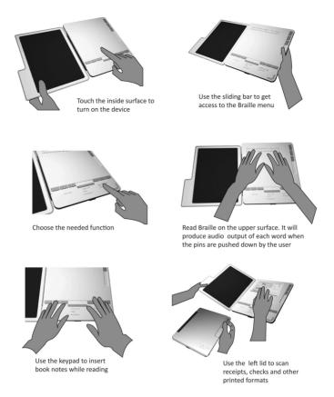
Figure 8.17 User experience storyboard for a new Braille reading device (illustration by Qian Yang)
