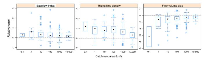
**FIGURE 5** Model bias error when a national model is used to simulate three signatures (baseflow index, rising limb density, flow volume), using data from 485 watersheds in New Zealand. These graphs are used to test hypotheses about how model performance varies with watershed area. Bias in all three signatures is lower for large watersheds (Reprinted with permission from McMillan, Booker, et al. (2016). Copyright 2016 Elsevier)
