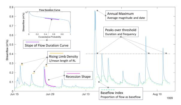
FIGURE 1 Examples of commonly used hydrologic signatures calculated as metrics of the streamflow timeseries
