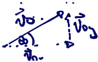
$$\left\{ \begin{array}{l} v_{0y} = v_0 \operatorname{sen} \theta_0 \\ v_{0x} = v_0 \operatorname{cos} \theta_0 \end{array} \right.$$
