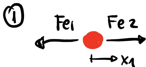
$$\Sigma F_x \quad -F_{e1} + F_{e2} = m \ddot{x}_1$$
