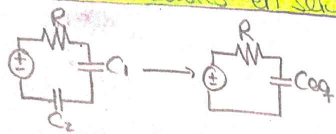
Donde  $C_{eq} = \frac{C_1 C_2}{C_1 + C_2}$
