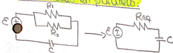
Donde  $R_{eq} = \frac{R_1 R_2}{R_1 + R_2}$
