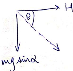
$$\begin{aligned} \theta &= \tan^{-1} \left( \frac{H}{mg \sin \alpha} \right) \\ &= \tan^{-1} \left( \frac{\sqrt{3} mg \sin \alpha}{mg \sin \alpha} \right) \\ &= 60^\circ. \end{aligned}$$
