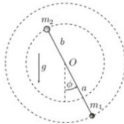
$$\vec{r}_1 = a \hat{\rho} \Rightarrow \vec{v}_1 = a \dot{\phi} \hat{\phi} // \vec{r}_2 = -b \hat{\rho} \Rightarrow \vec{v}_2 = -b \dot{\phi} \hat{\phi}$$
