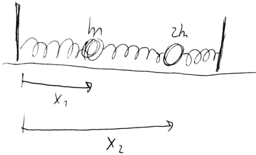
$$T = \frac{m\dot{x}_1^2}{2} + \frac{2m\dot{x}_2^2}{2}, V = \frac{k}{2}(x_1 - l_0)^2 + \frac{k}{2}(x_2 - x_1 - l_0)^2 \\ + \frac{k}{2}(3l_0 - x_2)^2$$
