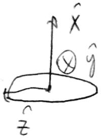
$$I_{cm}^{11} = \int_P (||\vec{r}||^2 \delta_{11} - \gamma_1 \gamma_1) dm \stackrel{r_i=0}{=} \int_P ||\vec{r}||^2 dm$$
