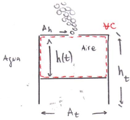
$$\rho_w = 1000 \frac{\text{kg}}{\text{m}^3} \quad A_h = 1 \text{ cm}^2 \quad h_t = 1 \text{ m}$$
