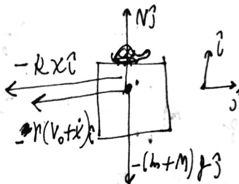
$$\ddot{X} + \frac{p}{m+m} \dot{X} + \frac{K}{m+m} (X + X_{\text{ef}}) = -\frac{\pi V_0}{m+M}$$
