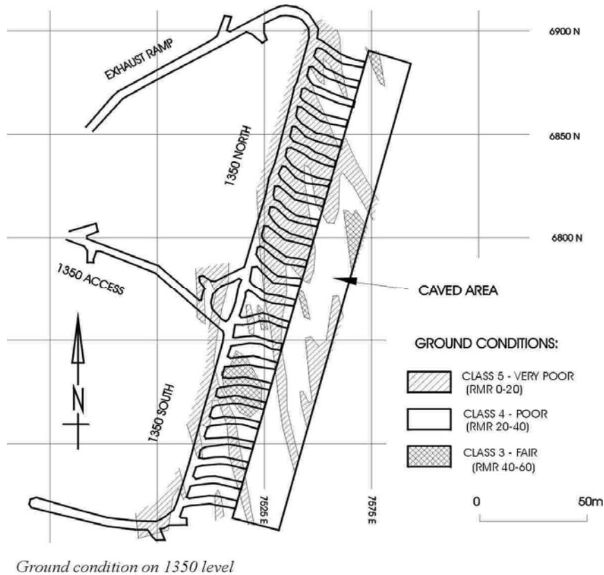
**Figure 2** Ground conditions at 1350 level
