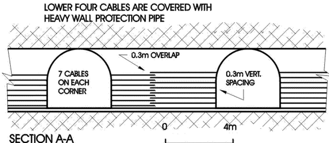
On some mines the cables have only been anchored in the drawpoint and then joined on the sidewall between the drawpoints. This is not advised as a long cable and does not provide good restraint owing to the greater elongation. The following photograph shows cables connected midway between the bullnose and camel back with the anchorage in the drawpoint.
