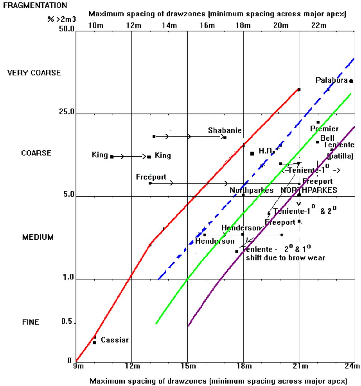
DIAGRAM SHOWING RELATIONSHIP BETWEEN MAXIMUM DRAWZONE SPACING AND CAVE FRAGMENTATION AND HOW THAT SPACING HAS BEEN INCREASED FOR DIFFERENT LHD OPERATIONS
