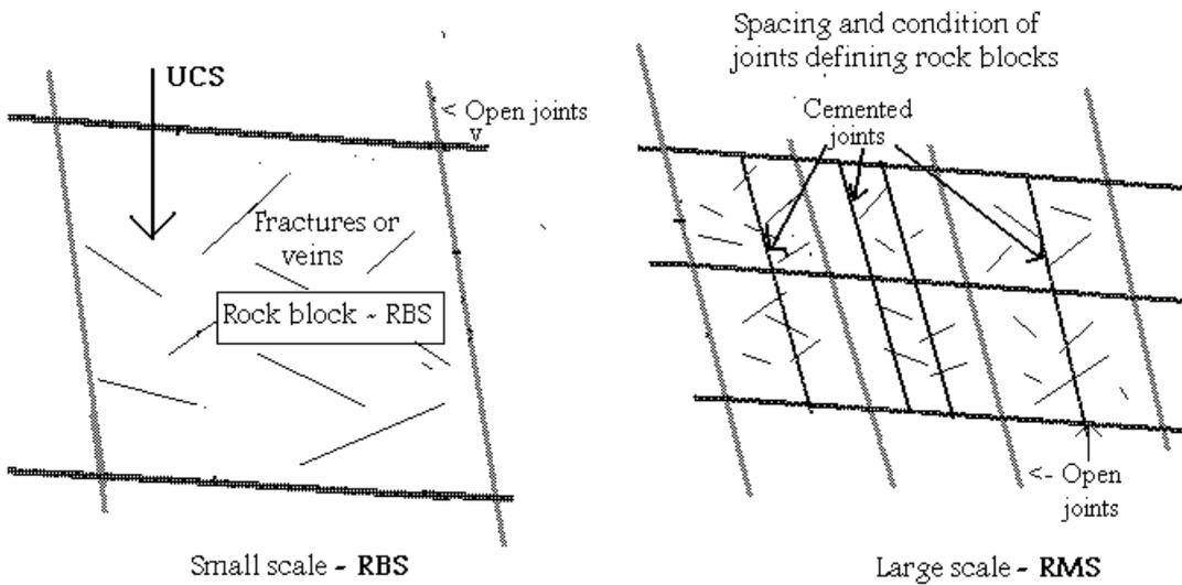
Figure 9. Diagrammatic representation of small scale RBS and large scale RMS
