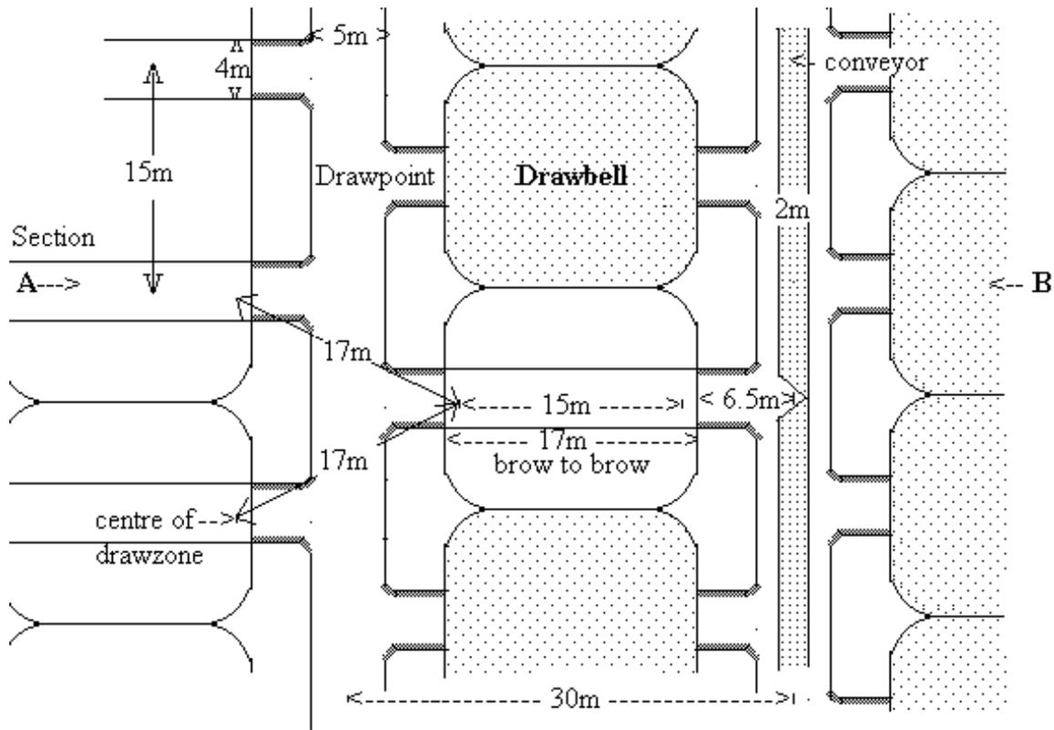
OFF-SET BACKHOE LAYOUT - DRAWZONE SPACING = 15m, 15m, 17m
