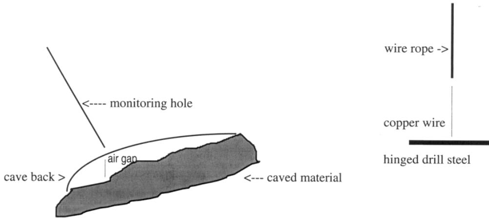
The drill steel is attached to the wire rope with a length of copper wire so that it can break easily when the back fails. The steel is lowered down the hole and pulled back to the cave back to measure the position of the back, it is then lowered to the broken rock and the height of the air gap established.
