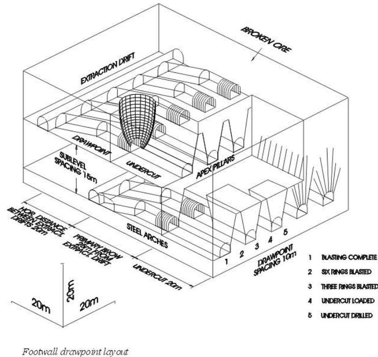
**Figure 3 Front cave layout. With undercut drill rings geometry**
