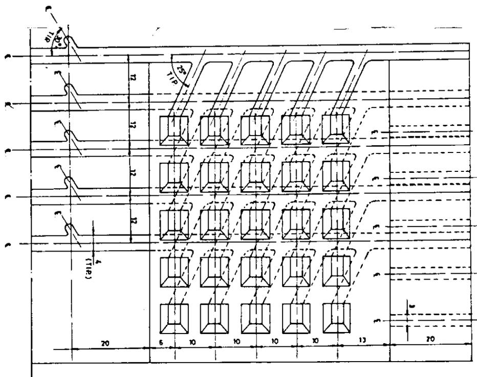
PLAN OF SUPERIMPOSED LEVELS AND DRAWBELLS IN AN EGGBOX LAYOUT
