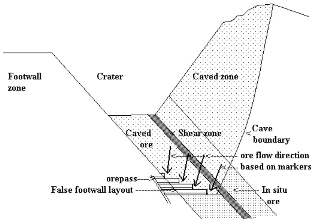
Diagrammatic section through King Mine showing Incline layout, major shear zone, caved zone and the direction of ore flow as determined by markers.
