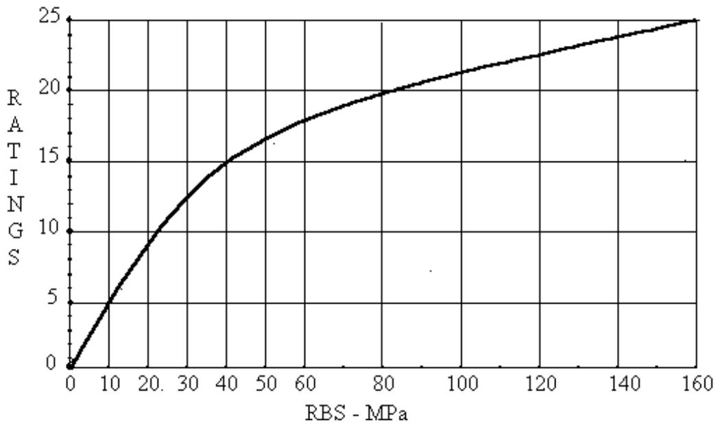
Figure 5. Rock block strength rating as a function of rock block strength.
