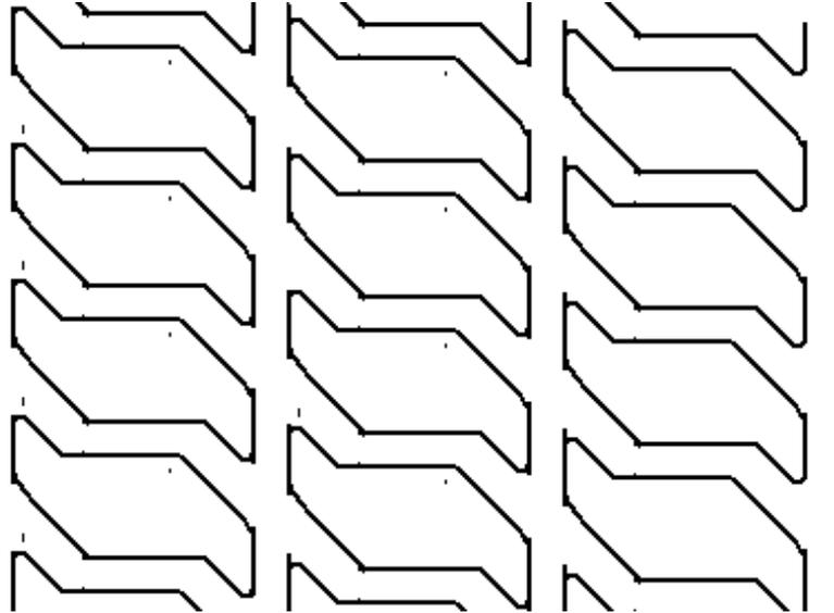
Parallelogram with drawpoints, drawbell drift and drawbells on same line at 60° to production drift.
