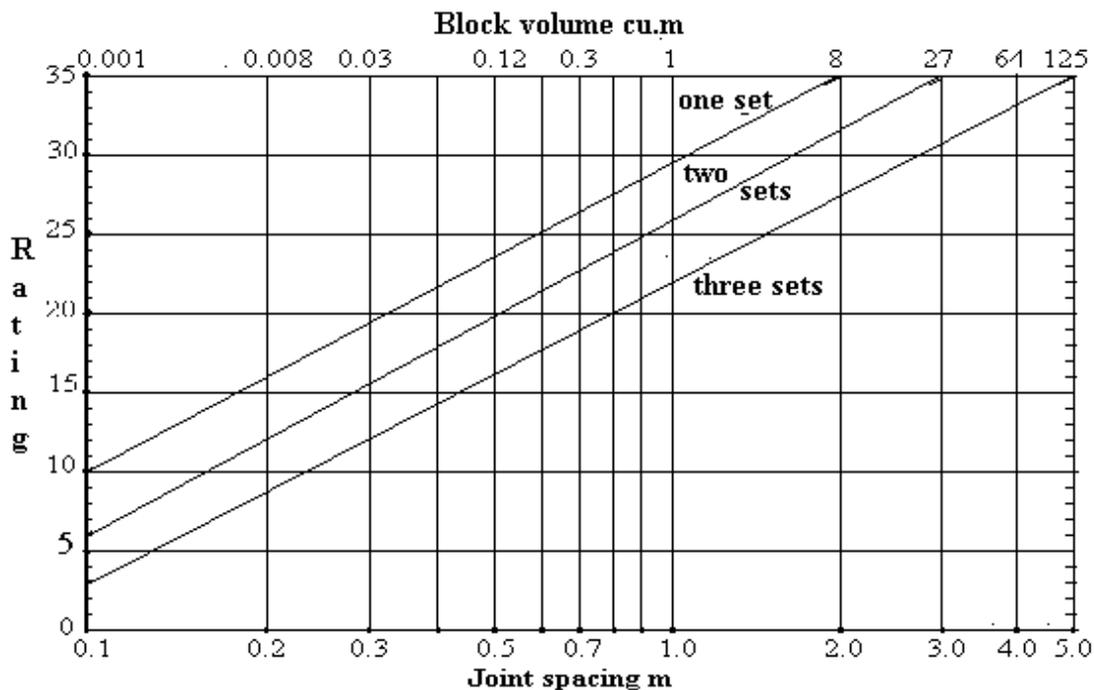
Figure 6. Joint spacing ratings
