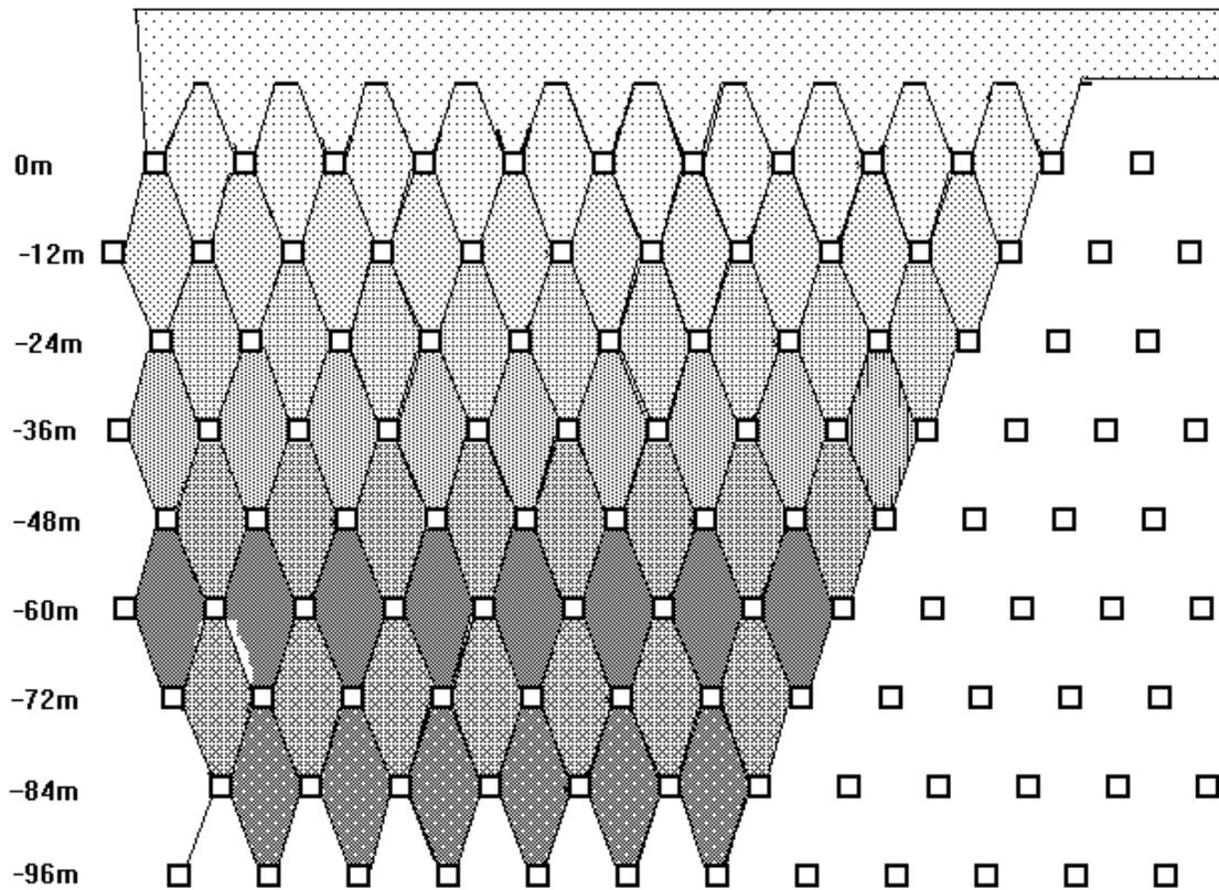
**End on view of Incline drawpoint layout showing brows of the drawpoints on levels 12m vertical interval and set back 15m from level to level.**
