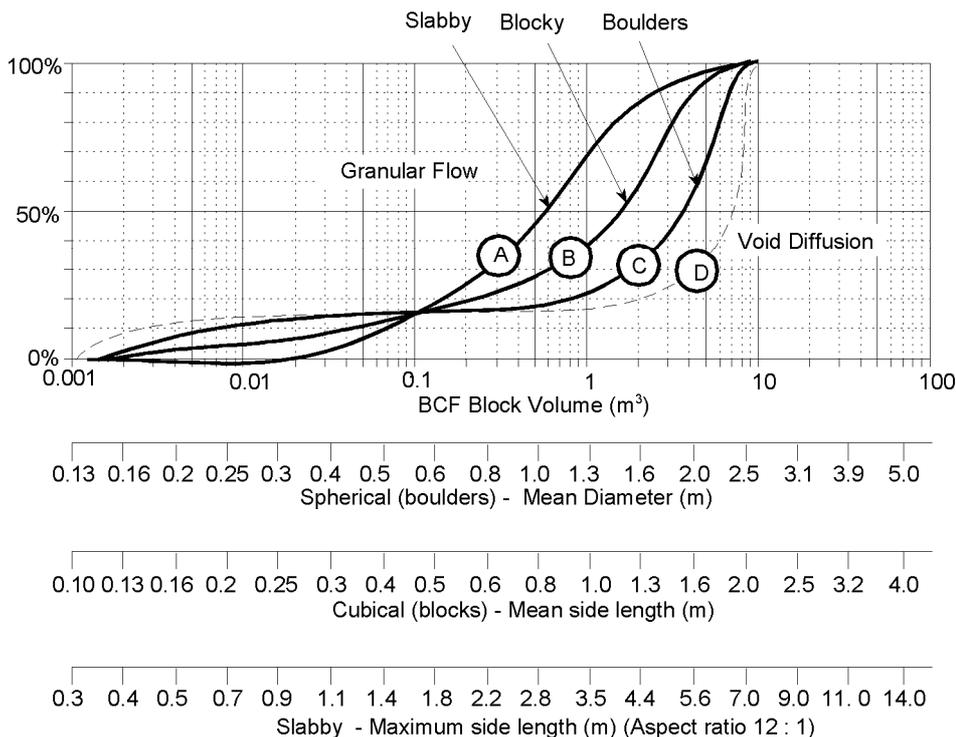
**Figure 9** | **Conceptual particle size distribution - draw mechanism relationship.**
