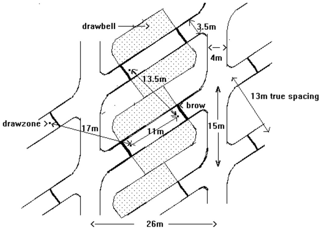
Drawpoints and drawbell drifts on same line at  $60^\circ$  to production drift. but, drawbells at right angles to production drift. Developed at Henderson Mine USA.
