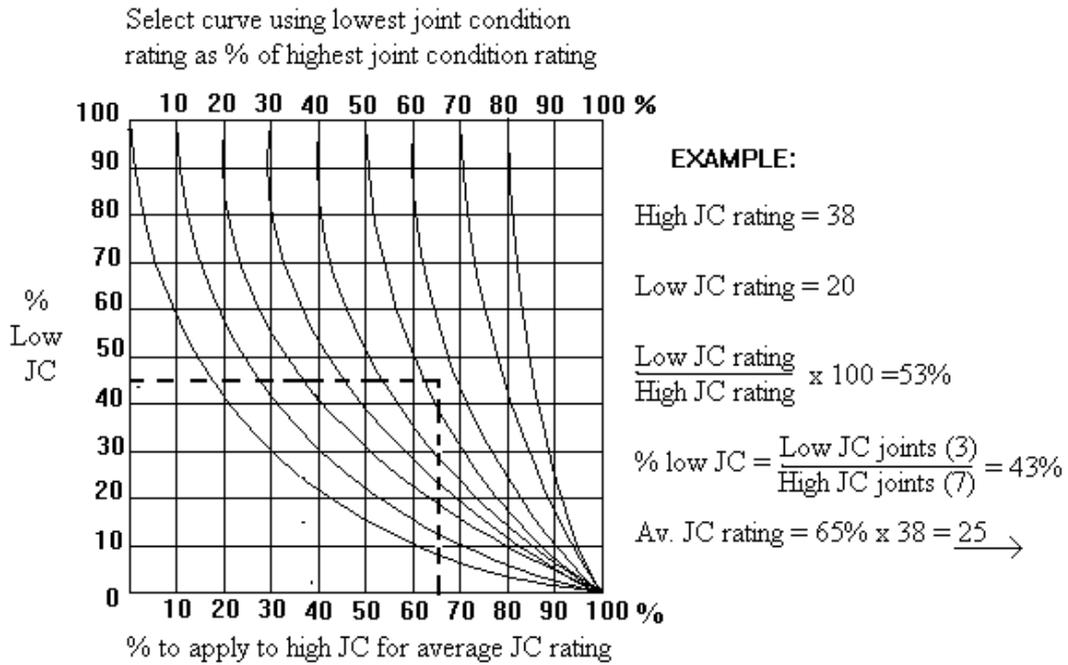
**Figure 8. Chart for averaging the joint condition for multiple joint sets.**
