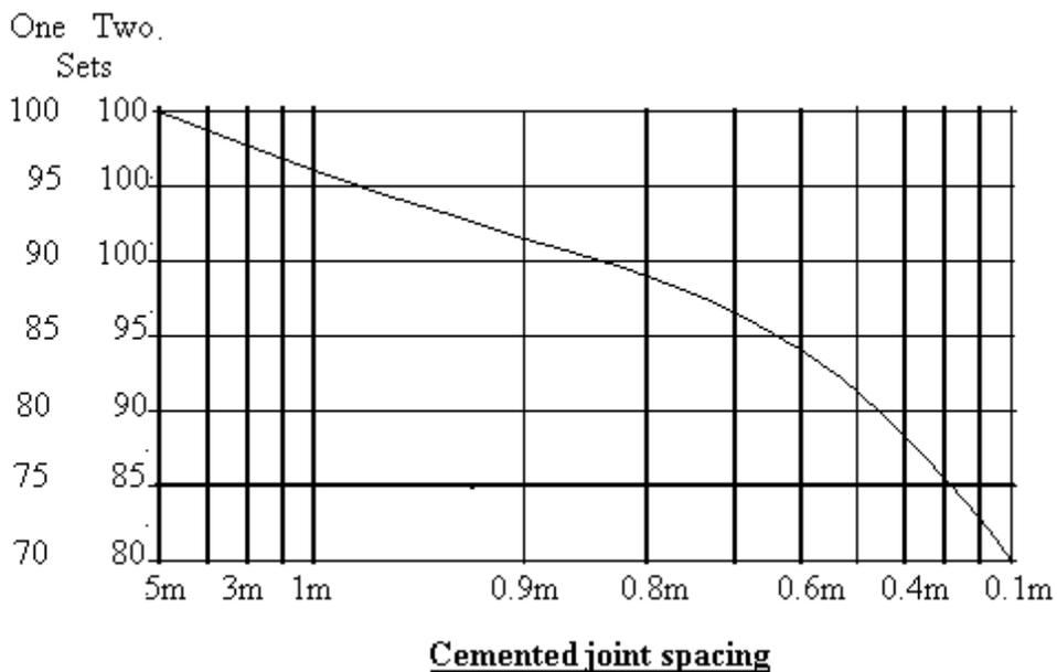
Figure 7. Adjustment factor for cemented joints
