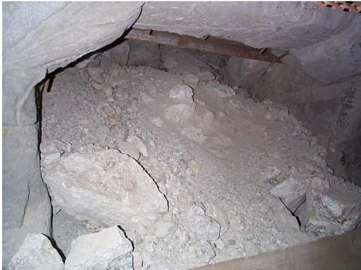
**Well fragmented ore flow controlled by board in bottom left of photograph**
