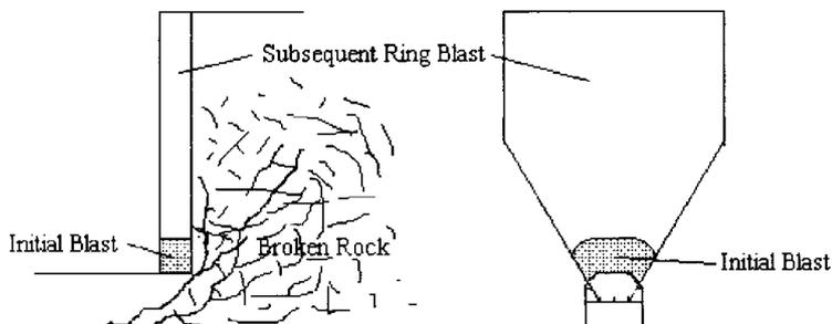
**Breaking of Rings in Two Sections when Relaxation Takes Place Near the Drift being Blasted**
