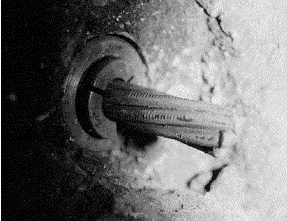
**Cable bolt pushing through the clamp**
