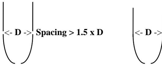
Sand model tests and the interpretation of stresses around underground excavations show that when the IDZ is spaced at more than 1.5 times the diameter (**D**) then there is no interaction. If the distance is less than  $1.5 \times D$  then there is interaction, the degree of which increases with reduction in spacing
