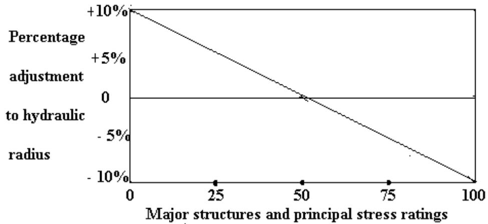
Figure 10. Adjustment factors for the effect of major structures on cavability
