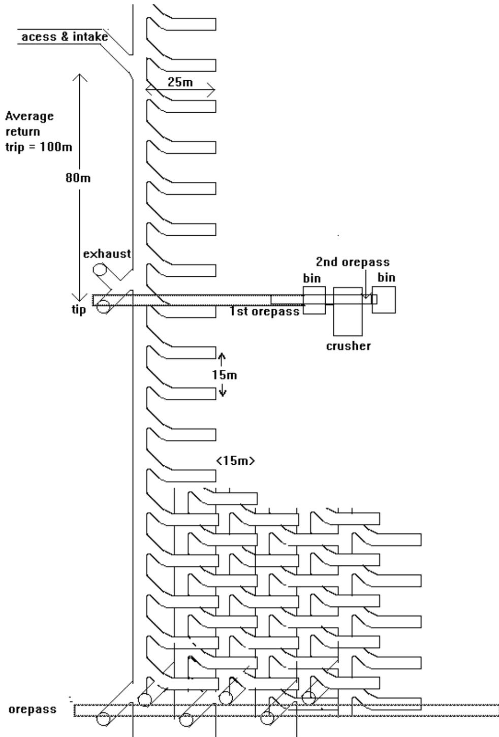
PLAN OF INCLINE DRAWPOINT LAYOUT - LEVEL INTERVAL 12M - DRAWPOINTS AT 15M
