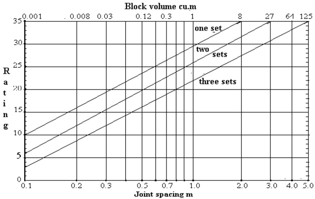
Figure 6. Joint spacing ratings
