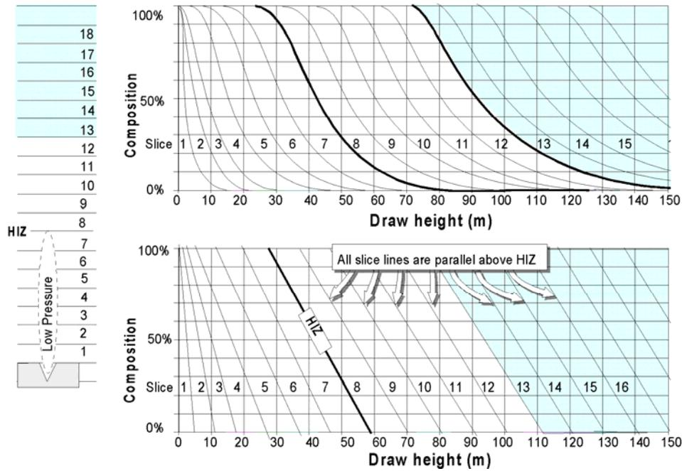
**Figure 16** Grade analysis graph for interactive draw. Top graph: Theoretical proportions Bottom graph: Simplified graph for manual grade calculations.
