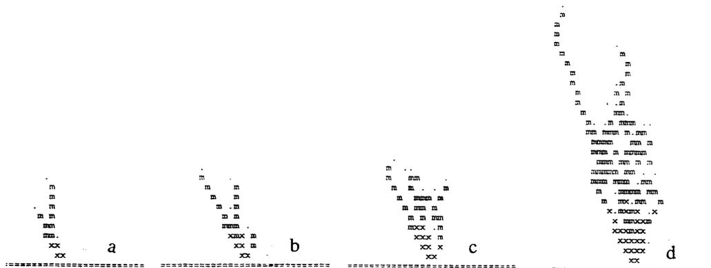
**Figure 5** Drawbody shapes from computer modelling. a: 6 blocks removed, b: 10 blocks removed, c: 16 blocks removed, d: 33 blocks removed.
