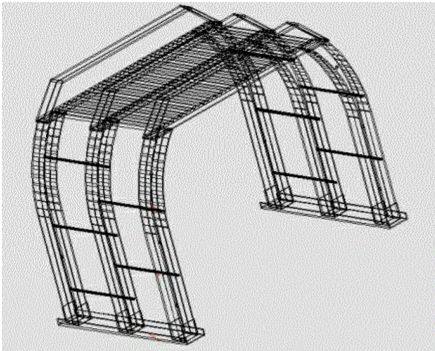
**Reinforced concrete lining** - A reinforced concrete lining was successfully developed at Bell Mine. Yielding steel arches were installed and backed with chicken mesh to act as a former. A reinforcing bar cage was installed between arch and sidewall and the opening filled with concrete. The inside of the arches are shotcreted for LHD protection.
