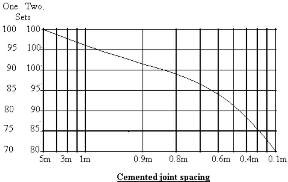
Figure 7. Adjustment factor for cemented joints
