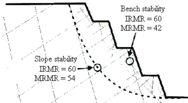
Figure 11. The difference in MRMR values used for bench and slope design.
