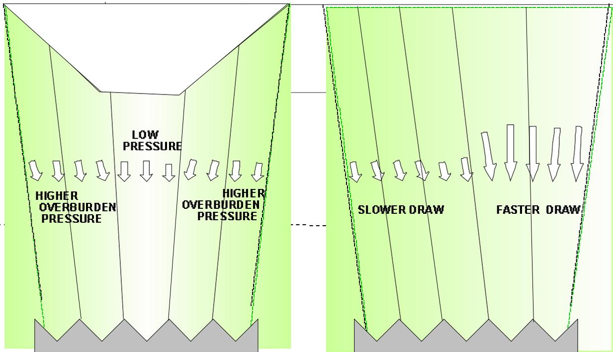
**Figure 13** Diagrams illustrating the inclination of draw columns towards higher pressure zones and areas of slower draw.
