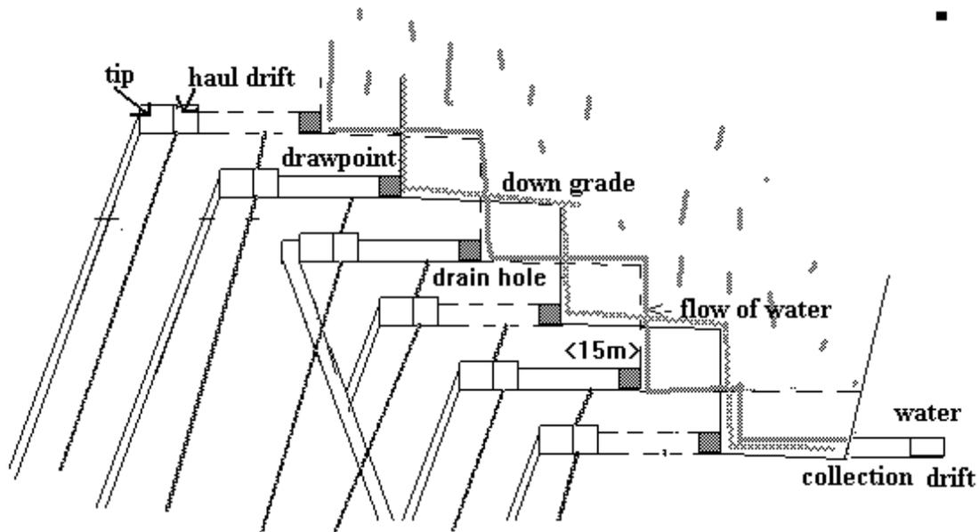
The same principles can be applied to the horizontal layout, particularly the drawpoints on the flanks if the water inflow is concentrated along the block boundaries.
