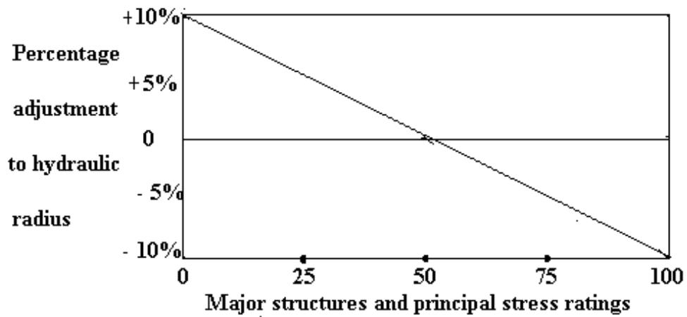
Figure 10. Adjustment factors for the effect of major structures on cavability
