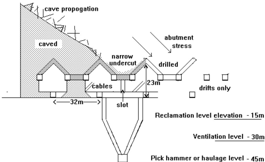
**Advance undercut with narrow incline and horizontal undercut, drawpoints and drawbell only developed after undercut has passed over so as to eliminate abutment stress damage. Cables installed from drawbell drift. Undercut holes angled forward, only limited swell relief with muck handled through orepasses in good ground at a slot site.**
