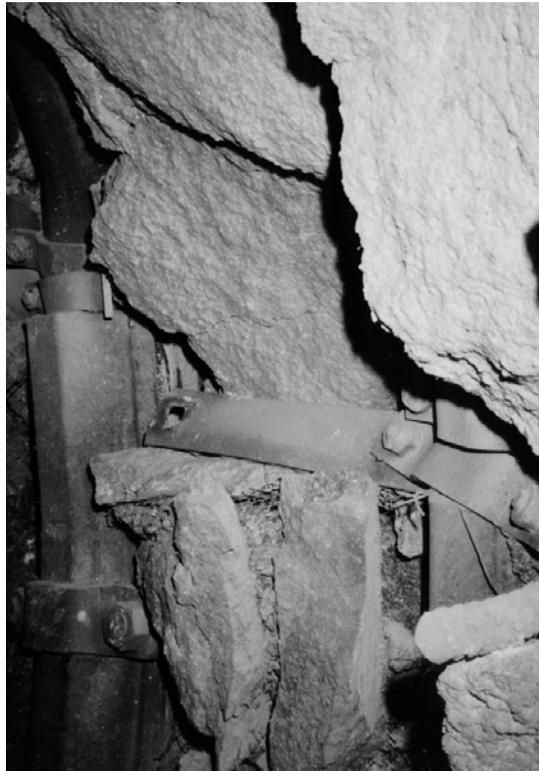
Figure 7b : Failed spacer between two arch legs
