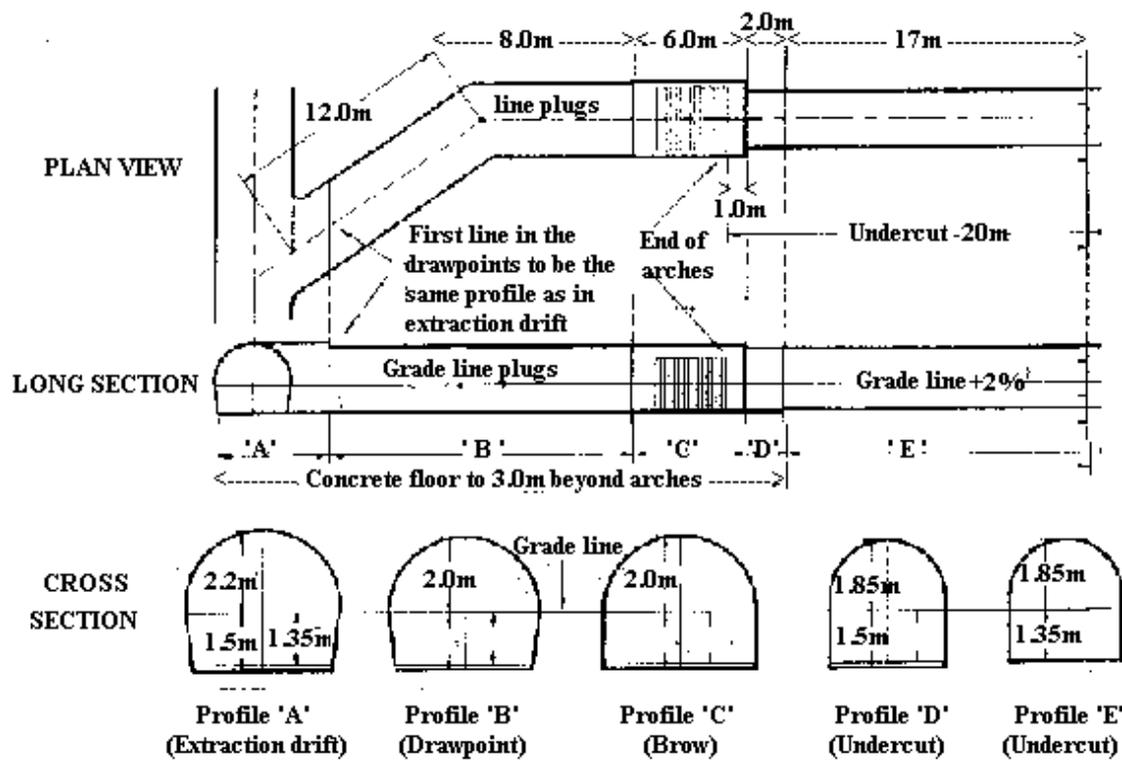
Figure 1 Geometry and excavation profiles of the drawpoints and undercut
