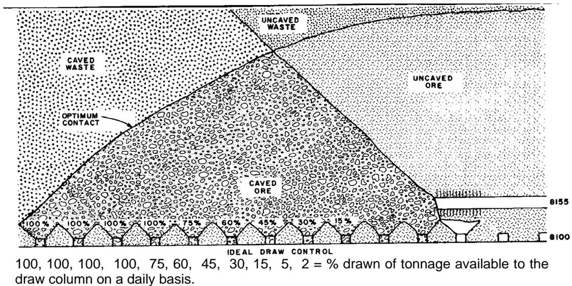
**Figure 11** Draw control with panel caving at Henderson Mine
