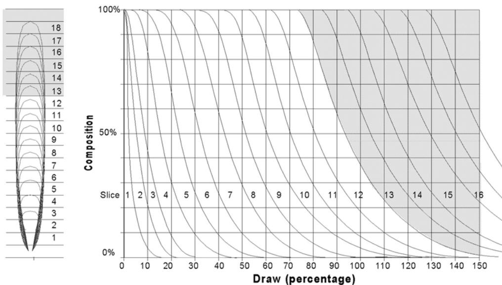
**Figure 14** Grade analysis graph for an isolated drawpoint in a granular material.
