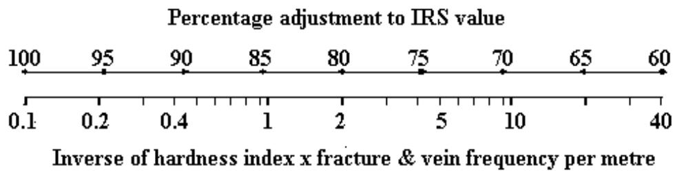
Figure 4. Nomogram for relating the IRS adjustment factor to the hardness index and fracture / vein frequency.
