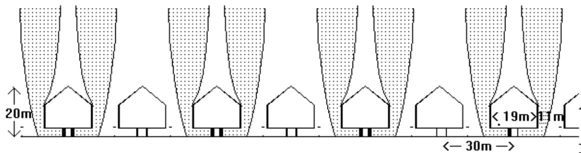
Figure 2 A - draw pattern of drawpoints either side of major apex i.e. from extraction drift
