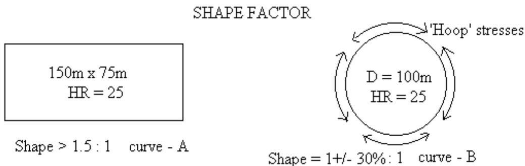
The following diagram shows two curves- curve A for rectangular orebodies and curve B for orebodies that are equi- dimensional.
