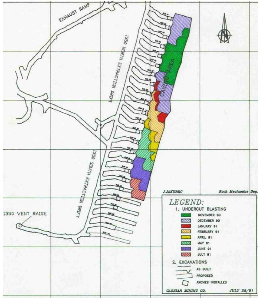
Figure 5 Undercutting sequence at 1350 level.
