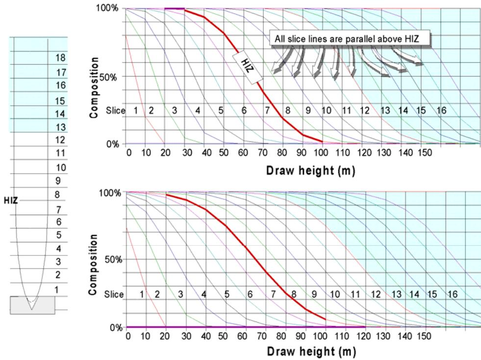
**Figure 15** Grade analysis graph for an isolated drawpoint in a VD draw. Top graph: Theoretical proportions Bottom graph: Simplified graph for manual grade calculations.
