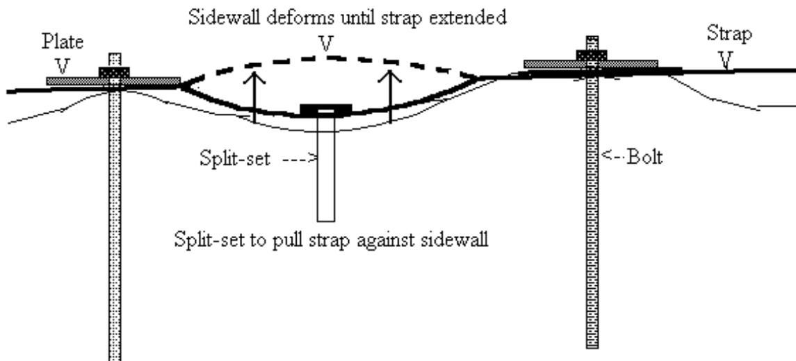
**Straps anchored against the wall rock with short split-sets**
