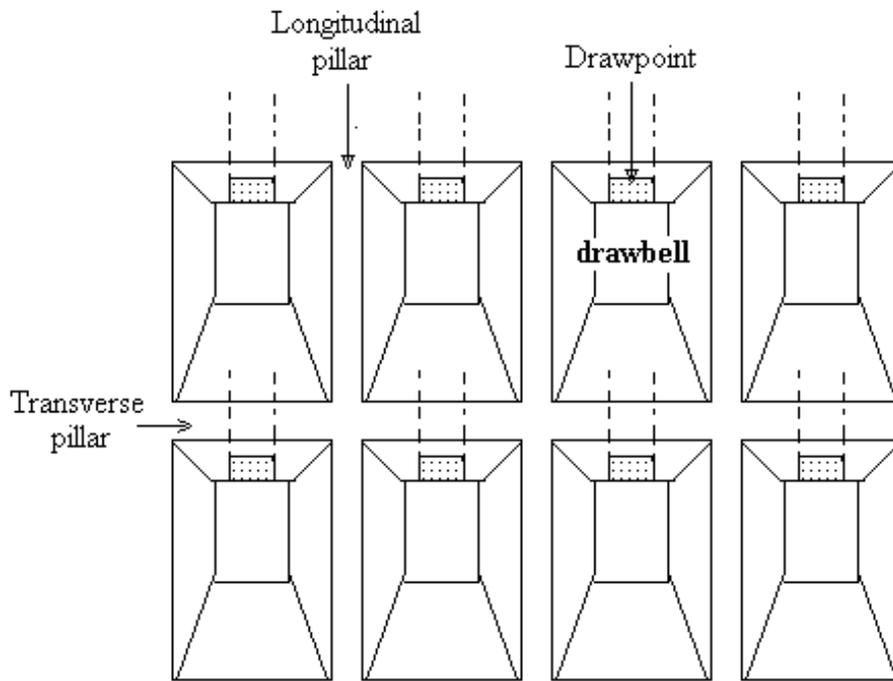
PLAN VIEW OF INCLINED EGGBOX LAYOUT
