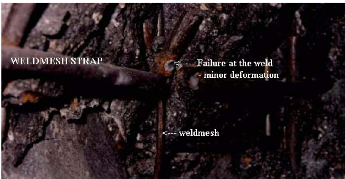
When weld mesh is subjected to deformation, the mesh fails at the welds with sidewall deformations of 50mm - this was readily observed at Cassiar mine under squeezing ground conditions. Chain link, however with 4.5mm diameter wire and 75mm openings was still providing support with deformations of 100mm. Chain link is available with wires of 5mm and openings of 50mm, 75mm and 100mm. It was surprising to read in a recent publication on support, that a 'leading authority' had condemned chain
