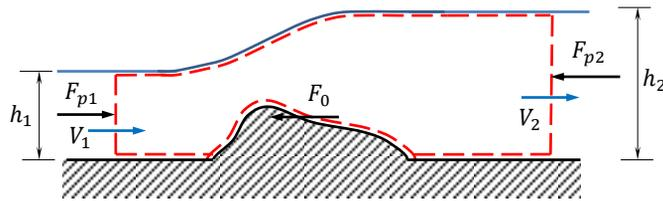
$$F_{p1} - F_{p2} - F_0 = \rho Q(\beta V_2 - \beta V_1)$$
