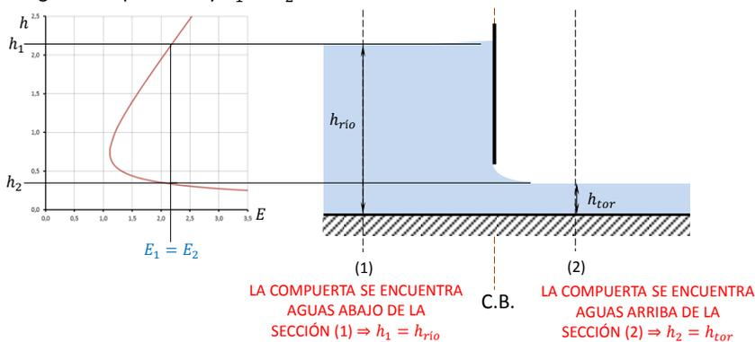
$$h_2 = \mu a \quad E_2 = \mu a + \frac{q^2}{2g(\mu a)^2} \quad E_2 = E_1 \quad h_1 + \frac{q^2}{2g(h_1)^2} = E_2$$
