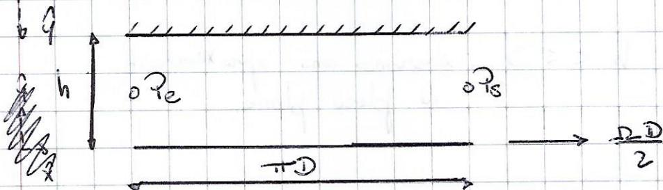
$$\boxed{1} \quad 0 = -\frac{\partial P}{\partial x} + \mu \frac{\partial^2 u}{\partial y^2}$$
