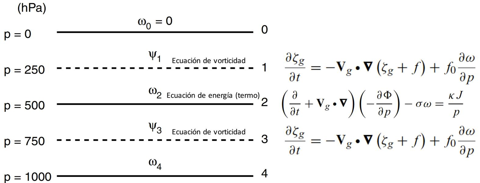
**Fig. 8.2** Arrangement of variables in the vertical for the two-level baroclinic model.
