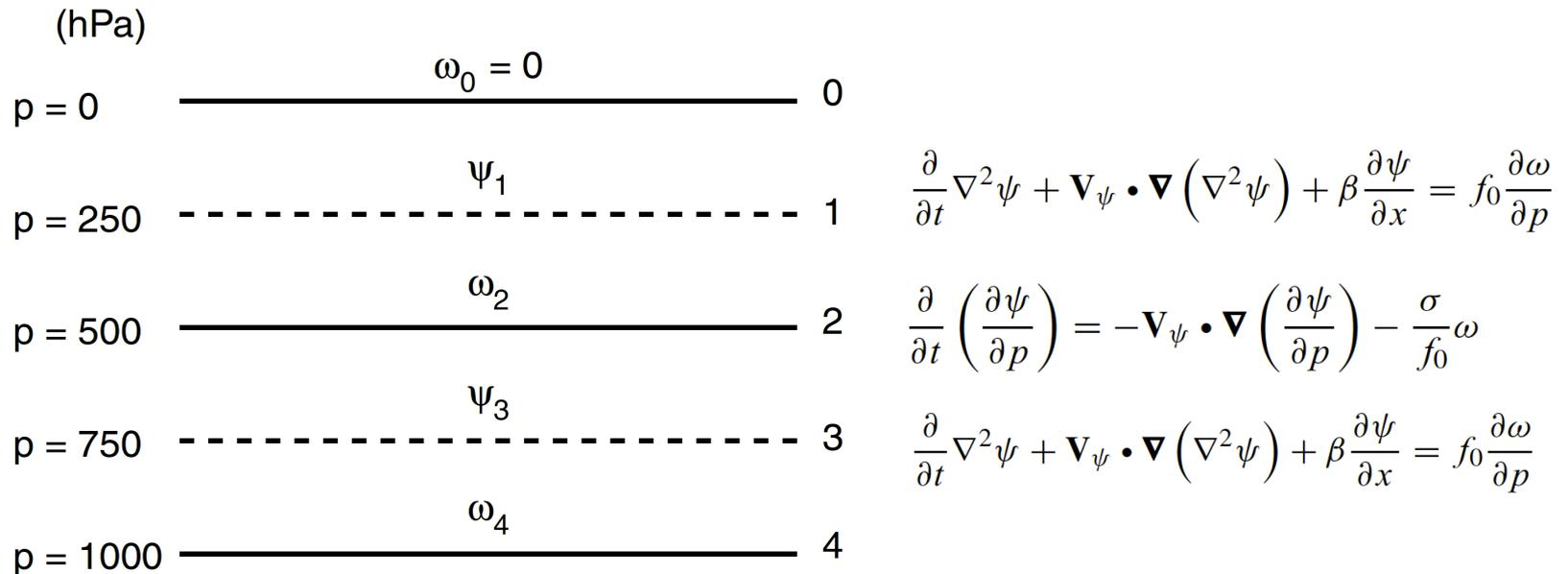
**Fig. 8.2** Arrangement of variables in the vertical for the two-level baroclinic model.
