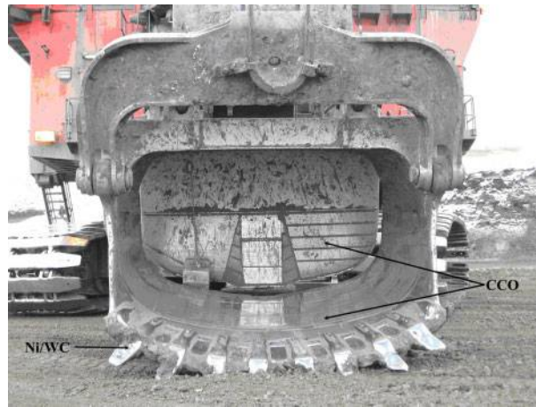
11 Bucket of electric rope shovel with both Ni–WC and CCO weld overlays 6
