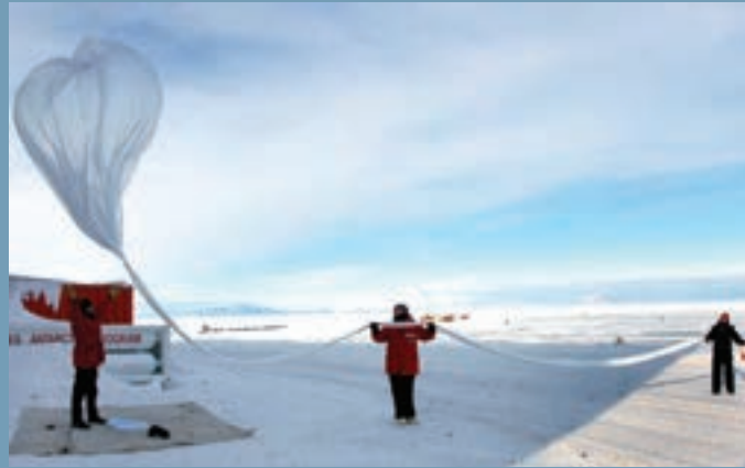
Scientists release a balloon from McMurdo Station in Antarctica carrying instruments that measure ozone depletion in the stratosphere.
