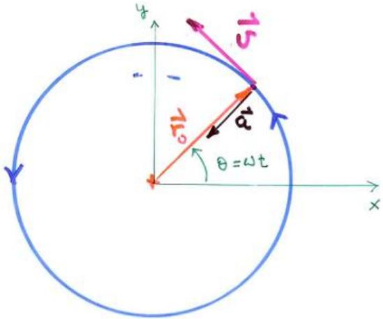
$$\vec{r} = [r_0 \cos \omega t, r_0 \sin \omega t]$$
