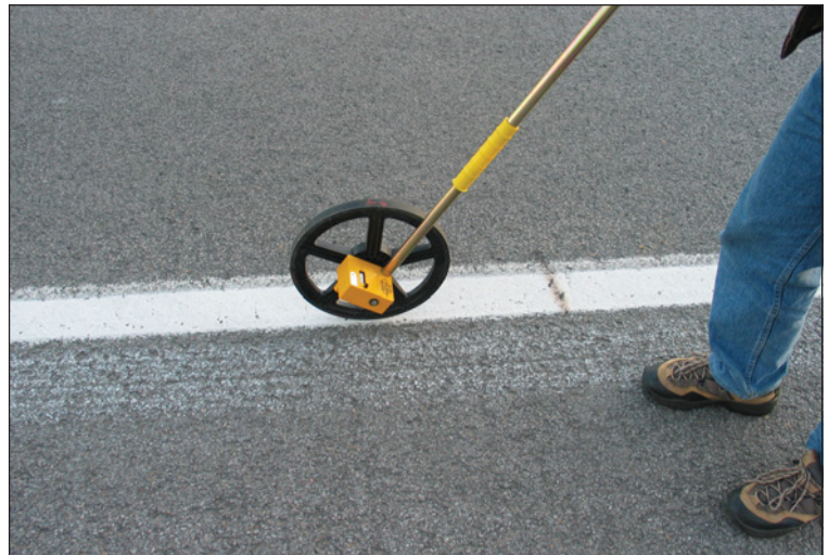
Measuring sight distance with a measuring wheel
