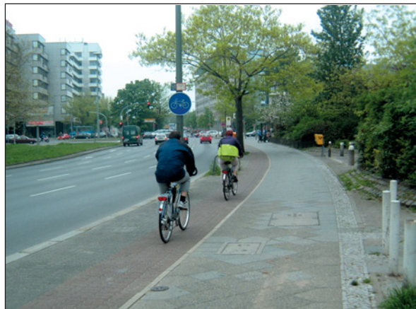
Urban arterials allowing proper separation of incompatible road users: wide and well-marked lanes, bicycle paths with different material and color and pedestrian traffic signals.
