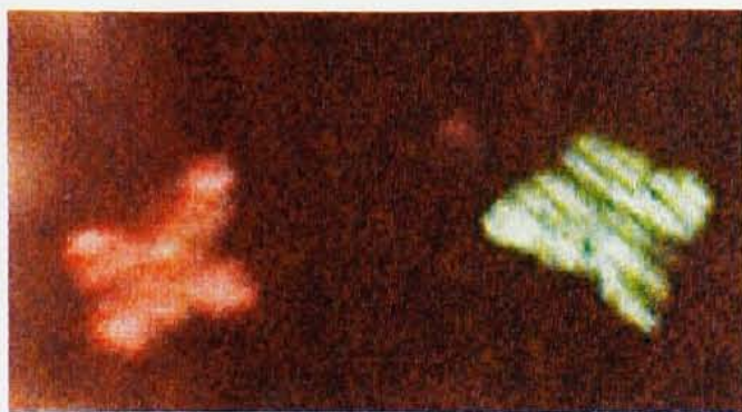
FIGURE 3. DENDRITIC GROWTH of crystallites of hard-sphere poly(methylmethacrylate) colloidal particles 508 nm in diameter at a volume fraction of \phi = 0.504 in a mixture of decalin and tetralin. Grown in microgravity on the space shuttle, the dendritic crystallites are 2–3 mm in diameter and persist for months. (Reprinted by permission from Nature , vol. 387, p. 883, copyright 1997, Macmillan Magazine Ltd.)
