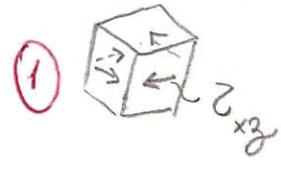
$\tau_{xz} = \frac{700 \text{ Nm} \times 0,03 \text{ m}}{J}$   $J = \frac{\pi d^4}{32} = 1,27234 \times 10^{-6} \text{ m}^4$
