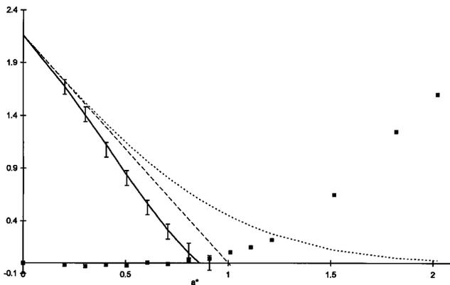
FIG. 1. The quantities  $N_s$  (squares) and  $g(\hat{r}, \phi)$  (bars) as defined in the text and determined by simulation as functions of the reduced shear rate. The bars indicate the estimated error in the latter quantity. The full line is from Eq. (5), the dashed line is from the linearization of Eq. (5), and the dotted line is the local-equilibrium contribution.
