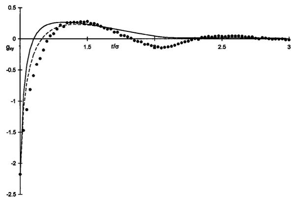
FIG. 2. The quantity  $g_{xy}(r)$  for reduced shear rate  $a^* = 0.5$ . The circles are from simulation, and the lines are from the calculation described in the text and based on Eq. (6). The full line uses the equilibrium value of  $v^*$  while the dashed line uses the value taken from the simulations.
