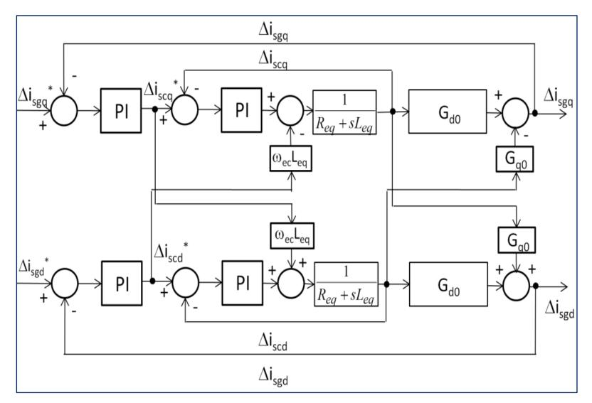
Nested control loops. The outer loop is regulating the currents of the power machine. The inner control loop is regulating the currents of the excitation machine.
