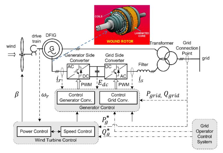
Power converters are usually designed for a nominal power of 30% of that of the doubly-fed machine.
