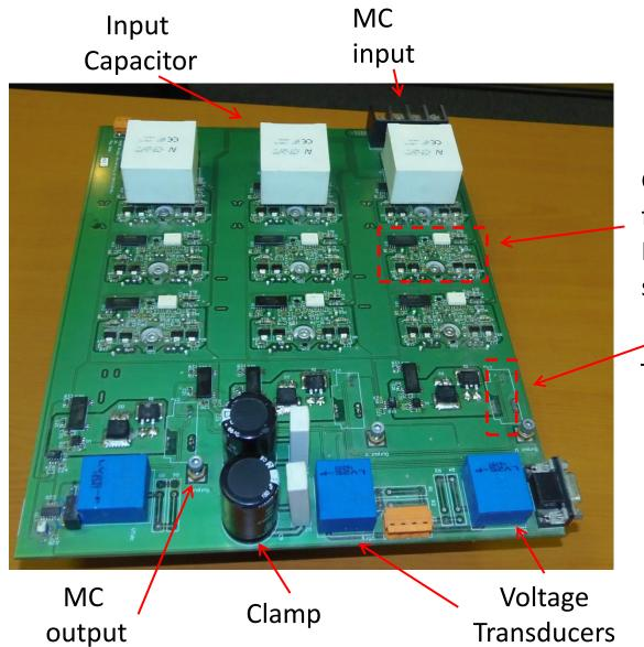
Gate Circuits for the Bidirectional switches Current Transducer
