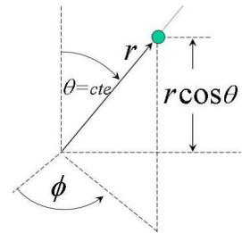
$$\text{En el instante final llega a } r_{\text{MÁX}} \Rightarrow \dot{r}_f = 0 \Rightarrow \frac{1}{2} m \frac{r_f^2}{2} \dot{\phi}_f^2 + mg r_f \frac{\sqrt{2}}{2} = 3mgH \quad (3)$$
