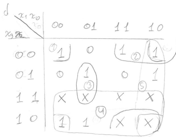
$$d = \bar{x}_2\bar{x}_0 + \bar{x}_2x_1 + x_2\bar{x}_1x_0 + x_3 + x_1\bar{x}_0$$
